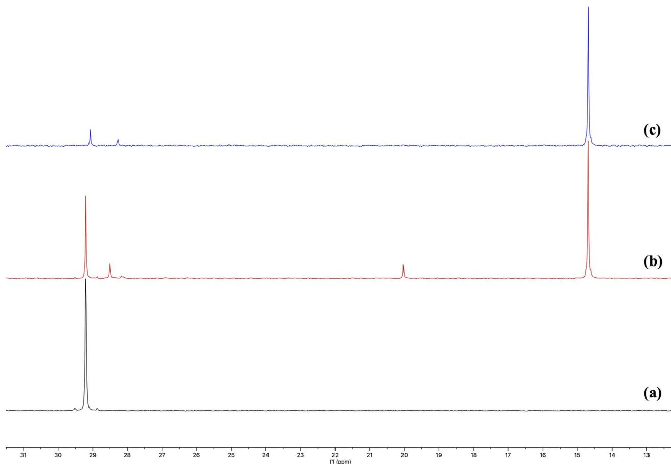
Fig. 4  $^{31}\text{P}\{^1\text{H}\}$  NMR spectra (162.0 MHz,  $\text{CDCl}_3$ , 298 K) of (a)  $\text{Pd}(\text{OAc})_2$  with  $2\text{PPh}_3$  milled for 2 hours with the formation of  $\text{PPh}_3\text{O}$ ; (b)  $\text{Pd}(\text{OAc})_2$  with  $2\text{PPh}_3$  milled for 30 minutes with the formation of  $\text{PPh}_3\text{O}$  and **4a**; (c)  $\text{Pd}(\text{OAc})_2$  with  $2\text{PPh}_3$  milled for 30 minutes in an Ar atmosphere with the formation of **4a** with high selectivity.
