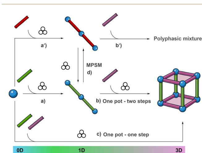
Fig. 1 Schematic representation of the experimental design followed for the construction of the PL-MOF. Path a or a': from a 0D to a 1D-CP (color code: Zn blue, **bipy** red, and **dpe** green); path b: from a 1D-CP to a PL-MOF (one pot – two steps; color code:  $\text{H}_2\text{ta}$  purple); path c: from a 0D to a PL-MOF (one pot – one step); path d: mechanochemical post-synthetic modification of 1D-CPs (linker exchange).
