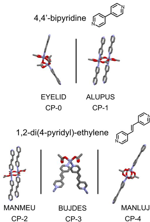
Fig. 2 Structures of the 1D-CPs obtained from  $\text{Zn}(\text{OAc})_2$  and **bipy** (top) or **dpe** (bottom). The naming refers to the CCDC ref. codes of the corresponding crystalline structures. Color code: Zn purple, N blue, O red, and C grey. Hydrogen atoms are omitted for clarity.
