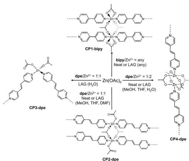
**Scheme 1** 1D-CPs mechanochemically synthesized and described in this work. The different linker/ $\text{Zn}^{2+}$  molar ratios and LAG agents are reported for each reaction. The water of crystallization of the metal salt has been omitted. See the Experimental section for details.
