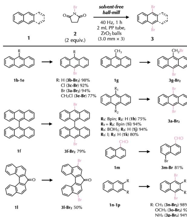
Fig. 4 Substrate scope in the mechanochemical reaction between **1** and **2** under solvent-free conditions. Yields determined by <sup>1</sup>H NMR spectroscopy with an internal standard. The experimental details for the isolation procedure and isolated yields for some of the products are described in the SI.
