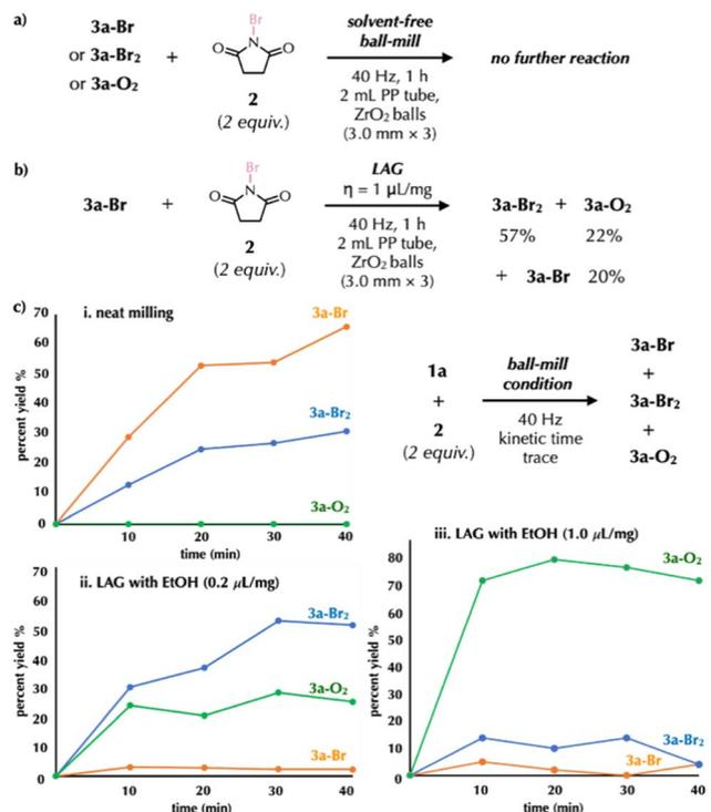
Fig. 2 (a) Control experiments of (a) solvent-free reactions between 3a-Br, 3a-Br<sub>2</sub> and 3a-O<sub>2</sub> and 2 and (b) a trace LAG reaction between 3a-Br and 2. (c) Reaction progress between 1a and 2 under different milling conditions: (i) solventless; and LAG with EtOH, (ii) 0.2 μL mg<sup>-1</sup> and (iii) 1.0 μL mg<sup>-1</sup>.
