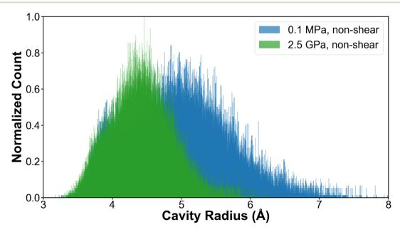
Fig. 6 Histograms of the cavity radius in the system at 0.1 MPa and 2.5 GPa without shear, computed over the last 0.5 ns of the NVT stage of the equilibration process.
