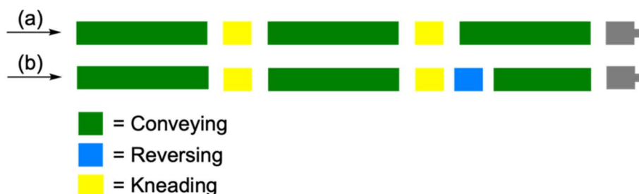
Scheme 11 Optimal extrusion condition for several examples of MCRs. (a) = Standard screw configuration for the first two reactions; (b) = alternative screw configuration for Petasis reaction.
