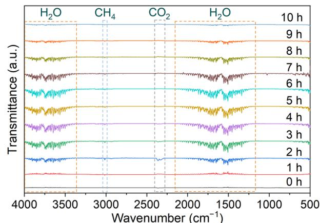
Fig. 4 Real-time FT-IR Spectra of the exhaust from milling NiO with a H<sub>2</sub> flow of 30 mL min<sup>-1</sup> at 100 °C.
