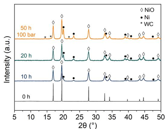
Fig. 1 XRD patterns of NiO powders milled for 0, 10, 20 h under 50 bar H<sub>2</sub> and 50 h under 100 bar H<sub>2</sub> in a planetary mill at room temperature.
