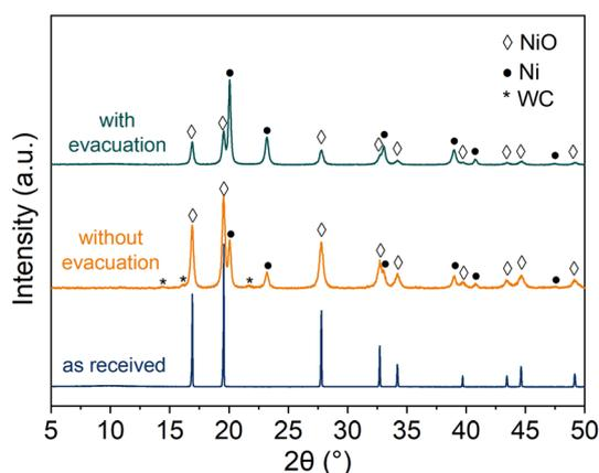
Fig. 2 XRD patterns of NiO powders milled under 100 bar H<sub>2</sub> for 50 h in a planetary mill, with and without evacuation sessions in between. Initial NiO is provided as reference.
