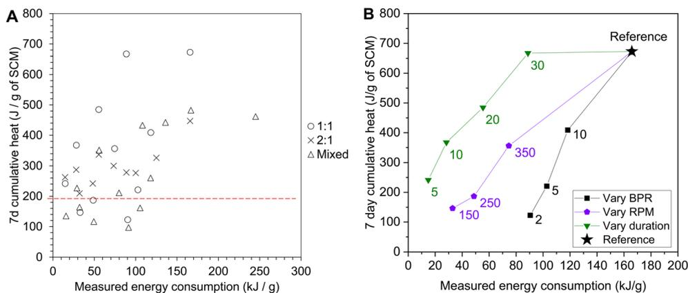
Fig. 5 (A) R<sup>3</sup> chemical reactivity vs. measured energy consumption for the data generated in this study. The dashed line at 190 J g<sup>-1</sup> of SCM corresponds to the threshold for a 'moderately reactive' activated clay.<sup>45</sup> (B) Datapoints for the 1 : 1 clay only, with each data series corresponding to the milling parameter being varied individually (same abbreviations as used in Fig. 4).
