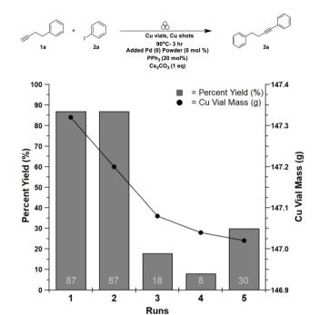
Fig. 2 Recyclability of palladium embedded in copper vial. Replicate reactions performed using a Cu ball (3/32''), Cu vial ( $2'' \times 0.5''$ ) with 3 hours of milling at 18 Hz and 90 °C using a Spex Certiprep 8000M.
