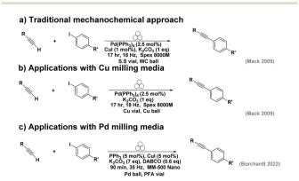
**Scheme 2** Explorations of the Sonogashira reaction driven by direct mechanocatalysis.
