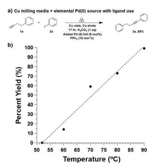
Fig. 1 (a) Mechanochemical Sonogashira using elemental palladium foil and triphenylphosphine at milling temperature (45 °C) and 17 hours of milling. (b) Mechanochemical Sonogashira using elemental palladium foil at various temperatures after 3 hours of milling.
