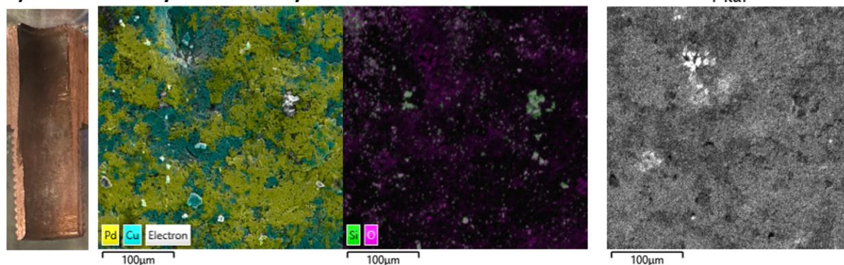
**Fig. 3** SEM-EDS chemical composition maps of the elemental species on (a) a brand new, unused copper vial, and (b) a copper vial utilized for a variety of reactions to test reaction substrate scope. More composition maps of other species observed on the vial utilized for a variety of reactions are available in SI 7.
