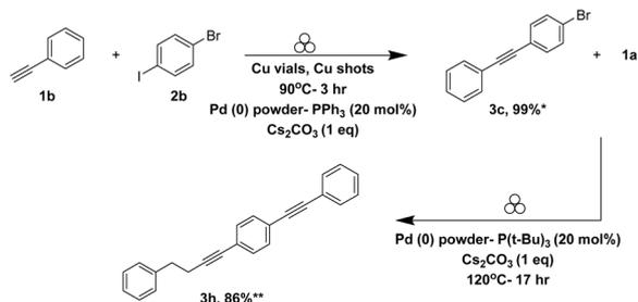
**Scheme 4** Tandem one pot mechanochemical Sonogashira reaction exploiting varying reactivity of iodine and bromine substituents. reactions performed using a Cu ball (3/32"), Cu vial (2" × 0.5") with milling at 18 Hz using a Spex Certiprep 8000M. \* Calculated as GCMS % conversion, \*\* Calculated as isolated yield.
