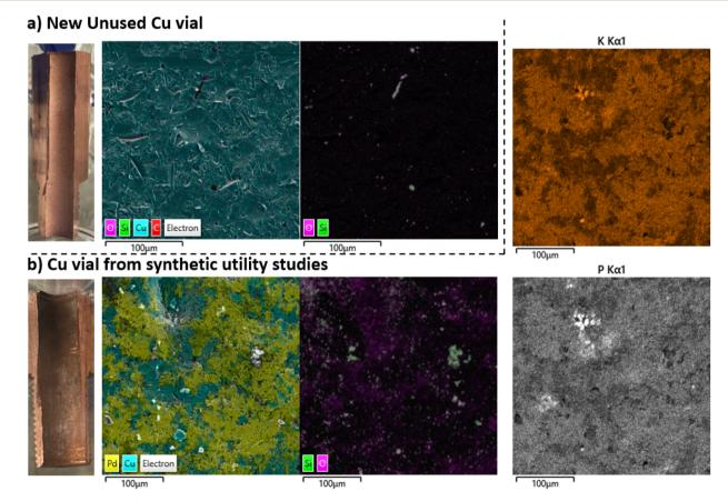
Fig. 3 SEM-EDS chemical composition maps of the elemental species on (a) a brand new, unused copper vial, and (b) a copper vial utilized for a variety of reactions to test reaction substrate scope. More composition maps of other species observed on the vial utilized for a variety of reactions are available in SI 7.
