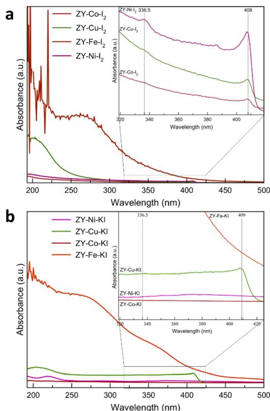
Fig. 4 Solid-state UV-Vis spectra of (a) ZY-M-I<sub>2</sub> and (b) ZY-M-KI samples (M = Fe, Co, Ni, Cu).
