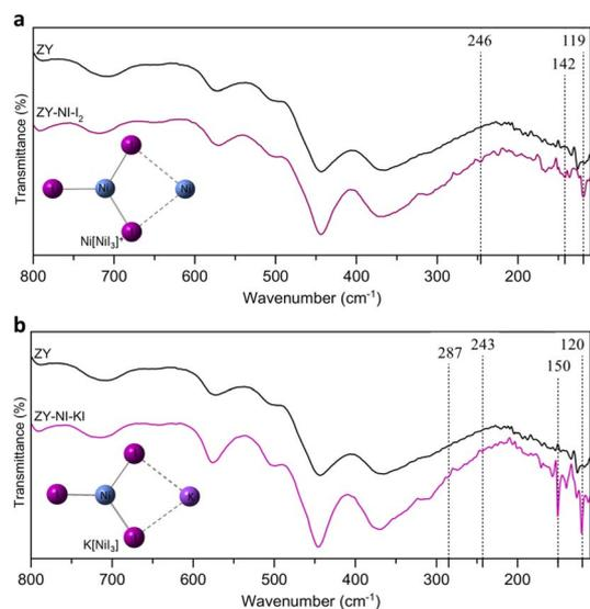
Fig. 3 Identification of iodide products *via* comparison of experimental far-IR spectra with calculated values. (a) Identification of Ni[Ni<sub>3</sub>]<sup>+</sup>. (b) Identification of K[Ni<sub>3</sub>]. The vertical lines denote vibrations present in the simulated spectra.
