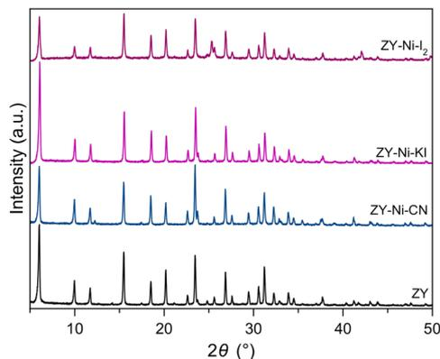
Fig. 1 PXRD patterns of the ZY-Ni samples milled with KCN/KI/I<sub>2</sub>.
