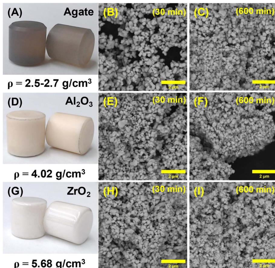
Fig. 4 Agate (A), corundum (D), and zirconia (G) milling media and corresponding SEM images of  $U_3O_8$  powder after milling for 30 min (B, E, and H) and 600 min (C, F, and I).
