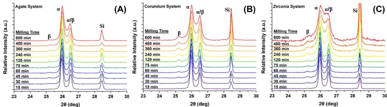
Fig. 3 PXRD patterns for  $U_3O_8$  samples milled with agate (A), corundum (B), and zirconia (C) milling media at 1167 rpm.
