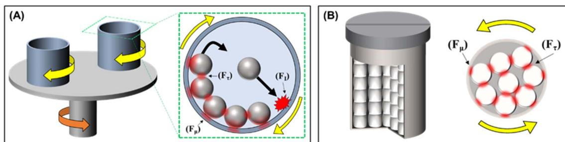
Fig. 8 Schematic of a planetary ball mill (A) and tumble mill (B).
