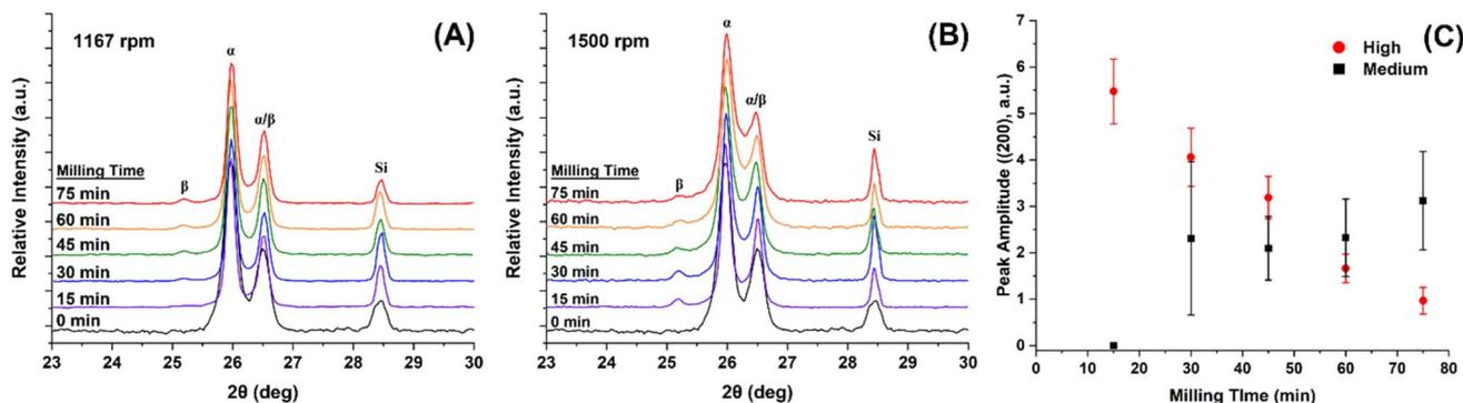
Fig. 2 PXRD patterns for  $\text{U}_3\text{O}_8$  samples milled with agate media at 1167 (A) and 1500 (B) rpm. Peak amplitudes of the (200)  $\beta$ - $\text{U}_3\text{O}_8$  diffraction peak ( $25.1^\circ 2\theta$ ) at high and medium milling speeds with increasing milling time (C).
