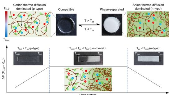
**P–N switchable thermoelectric ionogels enabled by microphase separation for intelligent thermal sensing**
