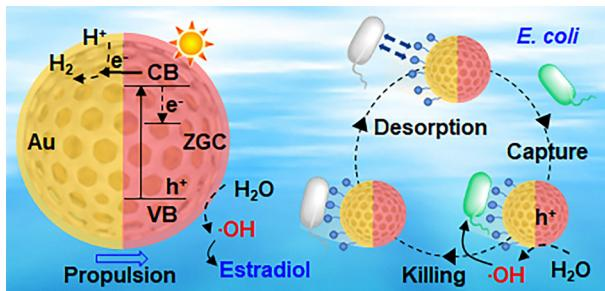
**Self-electrophoresis-propelled and self-built electric field-enhanced photocatalytic nanomotors for round-the-clock environmental remediation**
