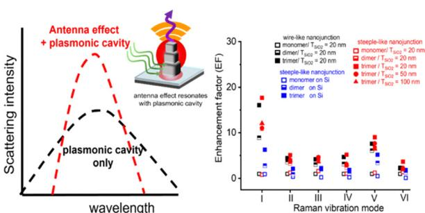
**Introducing plasmonic antenna nanojunctions into nanocavity structures to confine and enhance their local electromagnetic fields**
