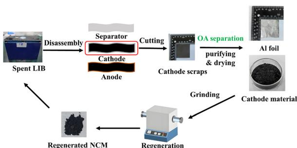
**Efficient separation of the NCM cathode material and Al foil from spent lithium-ion batteries with oxalic acid under mild conditions**
