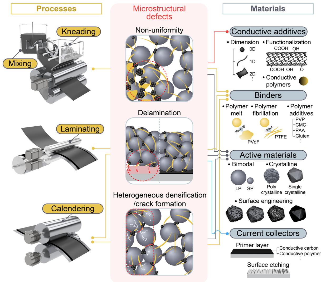
Fig. 2 Microstructural challenges in DPE manufacturing and the interplay between manufacturing processes and materials design.
