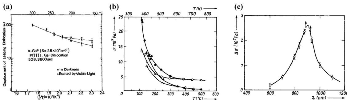
Fig. 10 (a) Temperature dependence of the radial displacement  $L$  of the leading Ga-edge dislocation in n-type GaP under indentation on the  $P\{\bar{1}\bar{1}\bar{1}\}$  surface. (b) Yield point ( $\sigma_y$ ) of n- and p-type GaAs crystals as a function of temperature under compressive deformation. (c) Spectral dependence of the illumination-induced stress reduction ( $\Delta\sigma$ ) in GaAs.<sup>22</sup> Copyright is from Wiley, Physica Status Solidi (a).<sup>22</sup>
