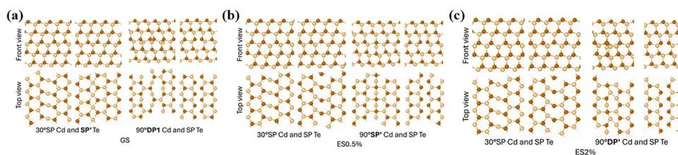
**Fig. 9** (a–c) Stable core structures of 30° and 90° Cd- and Te-core partial dislocations in CdTe under different excitation states: (b) ground state (GS), (c) ES0.5%, and (d) ES2%. Front- and top-view configurations are shown for each dislocation type. Cd and Te atoms are represented by yellow and orange spheres, respectively.<sup>52</sup> Copyright is from Elsevier, International Journal of Mechanical Sciences.<sup>52</sup>
