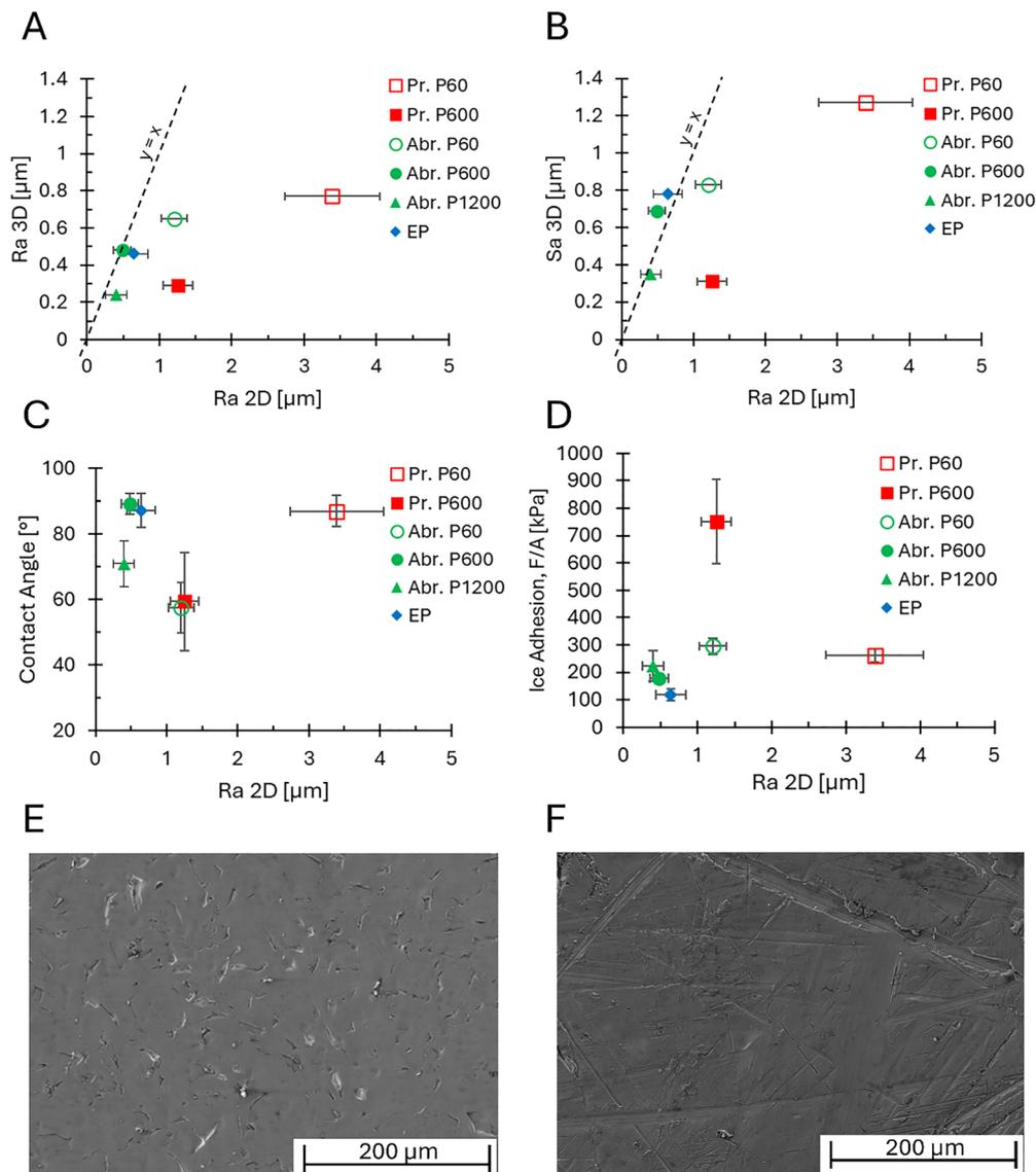
Fig. 4 (A) Average roughness values ( $R_a$ ) obtained using a 3D optical profilometer on a line profile and using a 2D stylus profilometer. (B) Average surface roughness values ( $S_a$  3D) against average profile roughness values ( $R_a$  2D) obtained using 3D optical and 2D stylus profilometers, respectively. (C) Contact angle versus  $R_a$  2D values. (D) Ice adhesion ( $F/A$ ) versus  $R_a$  2D values. The SEM images of (E) the "Pr. P600" sample and (F) the "Abr. P60" sample.
