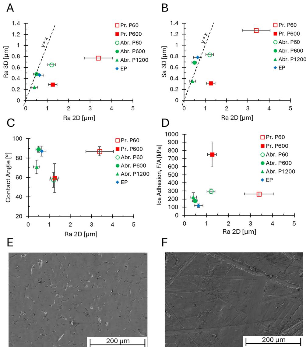
Fig. 4 (A) Average roughness values ( $R_a$ ) obtained using a 3D optical profilometer on a line profile and using a 2D stylus profilometer. (B) Average surface roughness values ( $S_a$  3D) against average profile roughness values ( $R_a$  2D) obtained using 3D optical and 2D stylus profilometers, respectively. (C) Contact angle versus  $R_a$  2D values. (D) Ice adhesion ( $F/A$ ) versus  $R_a$  2D values. The SEM images of (E) the "Pr. P600" sample and (F) the "Abr. P60" sample.
