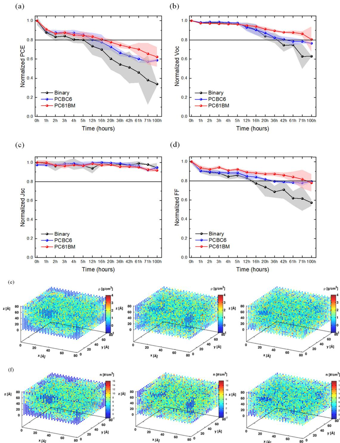
**Fig. 6** ISOS-D2-I thermal stability (85 °C inert atmosphere), normalized (a) PCE, (b)  $V_{oc}$ , (c)  $J_{sc}$  and (d) FF graphs. Solid lines correspond to the average values of  $N = 5$  individual cells for each blend, and the coloured area shows the deviation in each variation. (e) Heat maps of the mass and (f) number density of all system: left column (system 1), middle column (system 2) and right column (system 3).
