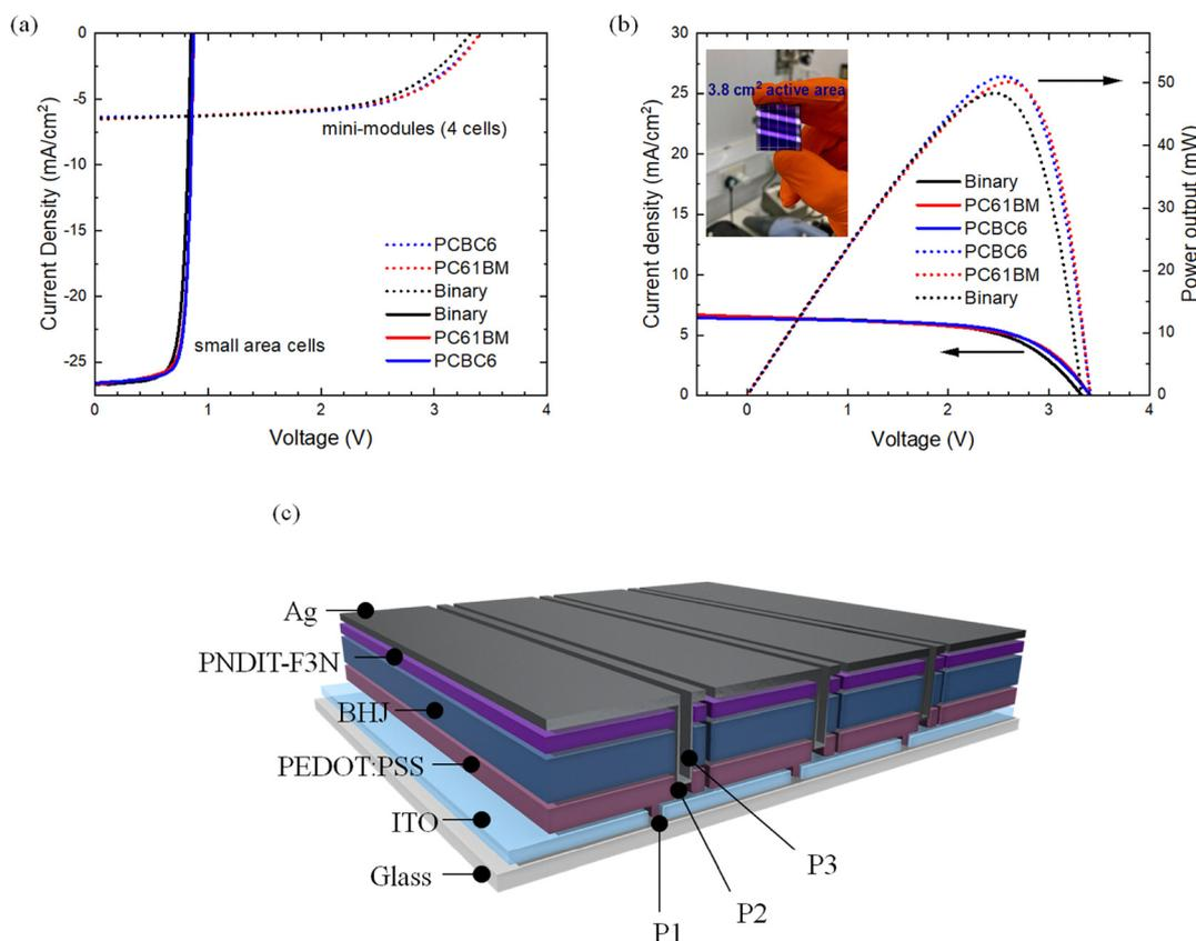
Fig. 7 (a)  $J$ - $V$  characteristics of mini modules (4 cells layout) and small area cells for binary ternary BHJ systems, (b) power output and current density-voltage curves for binary and ternary-based BHJ mini modules, and (c) schematic illustration of the solar mini modules (cross-sectional view).
