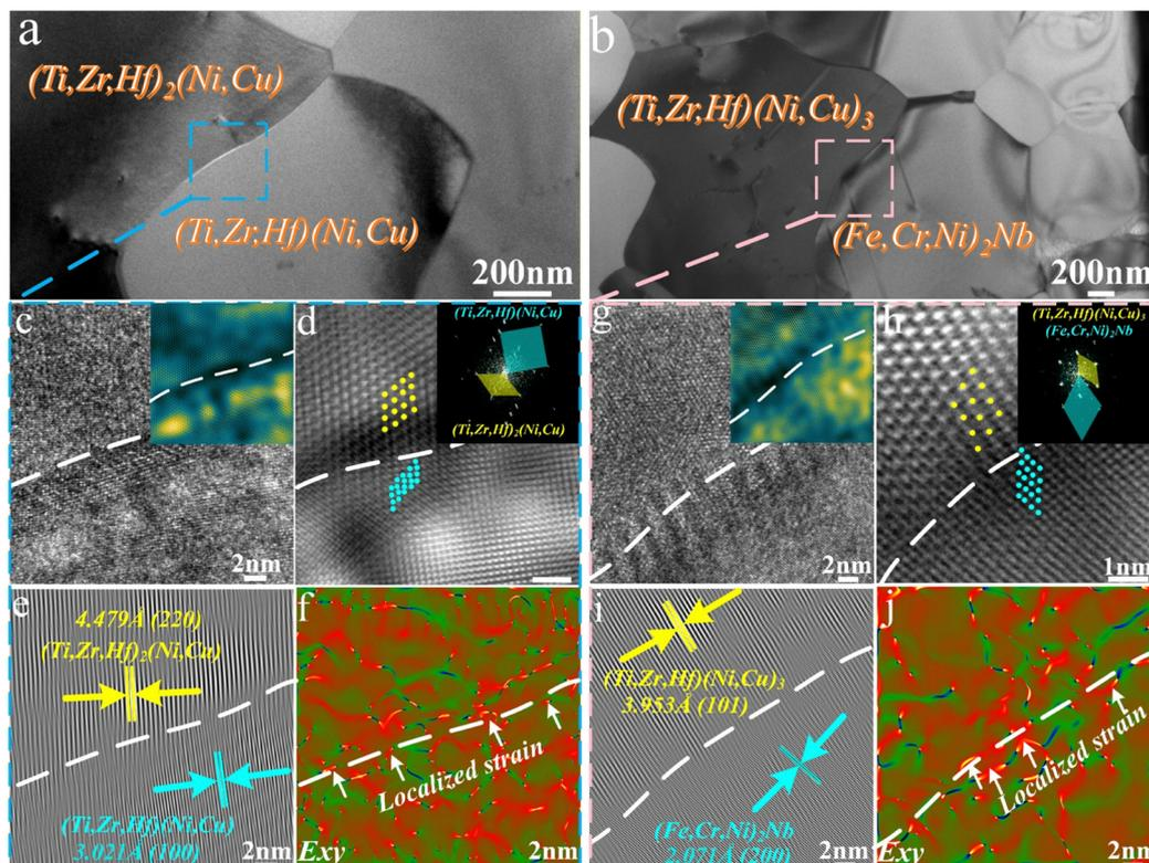
**Fig. 5** Interfacial characteristics of joints brazed at 1020 °C for 15 min with the HGFM. (a) and (b) Enlarged bright field images, (c) HRTEM image and lattice distortion conditions in (a), (d) FFT and lattice reconstruction image in (c), (e) lattice fringe image in (c), (f) shear strain distributions of (c), (g) HRTEM image and lattice distortion conditions in (b), (h) FFT and lattice reconstruction image in (g), (i) lattice fringe image in (g), and (j) shear strain distributions of (g).
