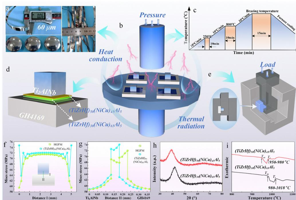
**Fig. 1** Innovative design of the brazing technique with the HGFM. (a) Brazing processing curve, (b) vacuum brazing diagram, (c) alloy ingots and foils, (d) assembly of brazing specimens, (e) shear test fixture, (f) and (g) residual stress along the horizontal and vertical directions for the brazed seam, and (h) and (i) XRD patterns and DSC curves of the HGFM.
