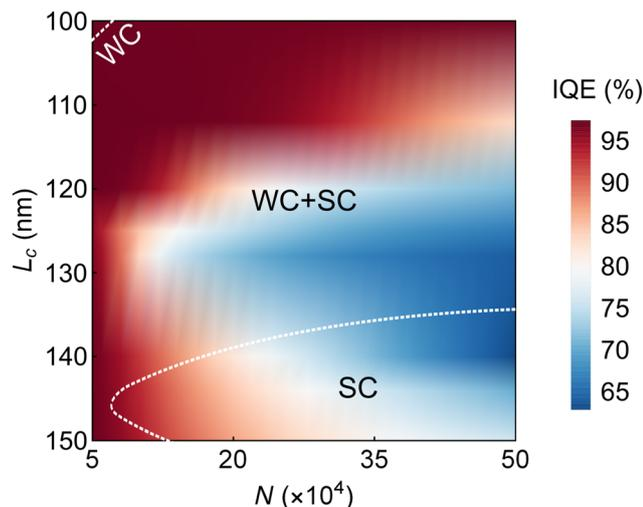
Fig. 4 IQE as a function of cavity thickness  $L_c$  and the number of coupled molecules  $N$ . The white dashed curves separate regions, where the system is entirely in the weak-coupling regime (WC), strong-coupling regime (SC), or different regimes at different outcoupling angles (WC + SC).
