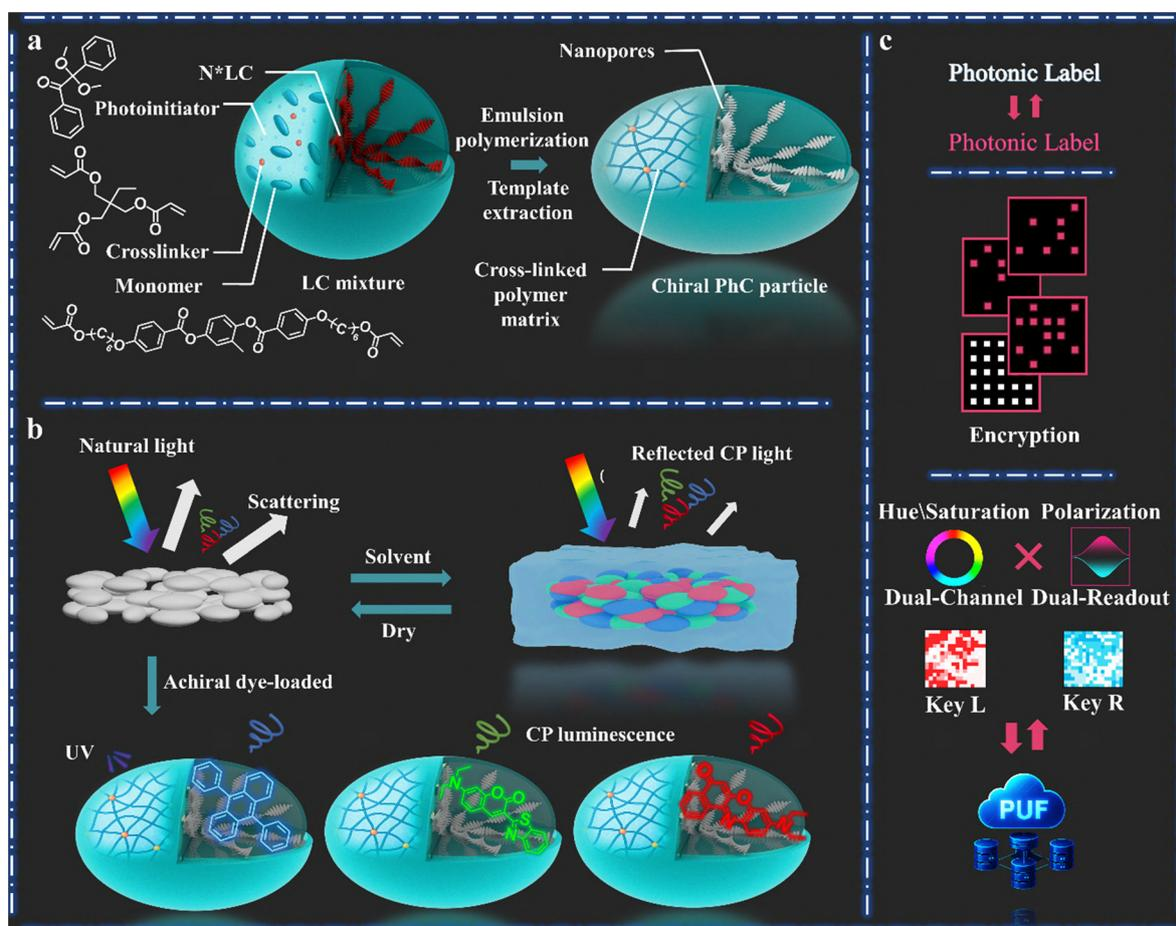
**Fig. 1** Scheme illustration of (a) the fabrication process of chiral PhC particles, (b) the “off-to-on” switching mechanism driven by scattering modulation, which can be further extended to dye-loaded systems to achieve CP luminescence and (c) chiral PhC particle applications: photonic label (top), encryption (middle), and physical unclonable function (bottom).
