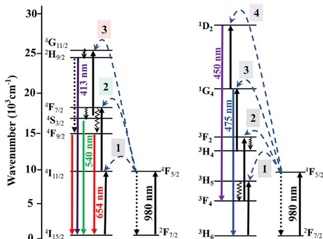
Fig. 4 Energy level diagrams of  $\text{Er}^{3+}$  and  $\text{Tm}^{3+}$  ions illustrating the upconversion pathways responsible for green ( $\sim 540$  nm), red ( $\sim 654$  nm), blue ( $\sim 475$  and  $450$  nm), and violet ( $\sim 413$  nm) emissions under  $980$  nm CW excitation. The labeled transitions correspond to two-, three-, and four-photon processes that enable sequential RGB tuning.
