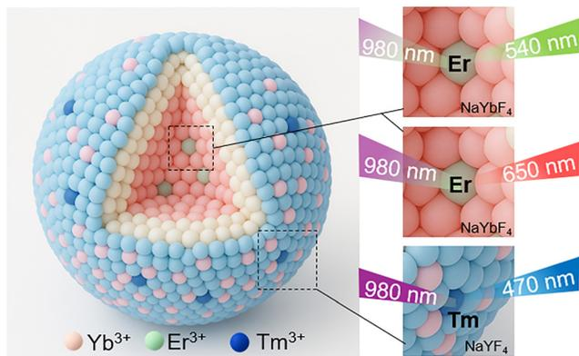
Fig. 1 Schematic of the core/shell/shell (C/S1/S2) nanocrystal with a  $\text{NaYbF}_4:\text{Er}^{3+}$  core, inert  $\text{NaYF}_4$  intermediate shell, and  $\text{NaYF}_4:\text{Yb}^{3+}, \text{Tm}^{3+}$  outer shell, enabling power-dependent RGB emission tuning under CW 980 nm excitation.
