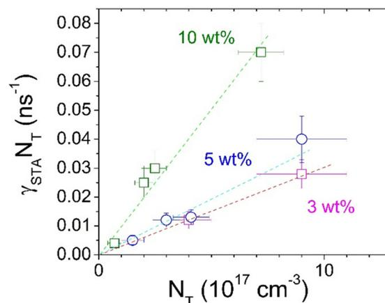
Fig. 4 Rate constant of PL quenching vs. steady state triplet density  $N_{\text{T}}$  determined using the data shown in Fig. 3, Fig. S4 and S6. The dashed lines are linear fits used for determining  $\gamma_{\text{STA}}$ .
