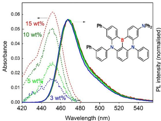
Fig. 2 Absorbance (dashed lines) and normalized PL ( $\lambda_{\text{exc}} = 375$  nm) spectra of DABNA-2 dispersed in mCBP host at different concentrations in wt%. The inset shows the molecular structure of DABNA-2.
