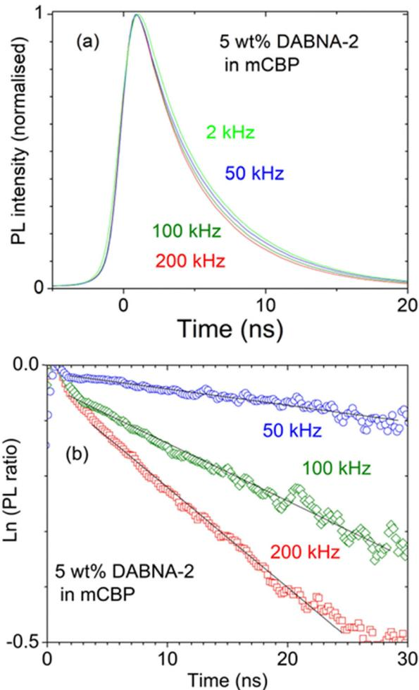
Fig. 3 (a) Kinetics of the DABNA-2 prompt fluorescence in film with 5 wt% of DABNA-2 in mCBP measured with varying  $f_{\text{rep}}$  of excitation pulses at 343 nm at an incident pulse density of  $5 \mu\text{J cm}^{-2}$ . (b) Natural logarithm of the PL ratio =  $I(\text{high } f_{\text{rep}})/I(2 \text{ kHz})$  (symbols) and fits to eqn (3) (solid lines).
