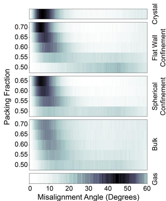
**Fig. 5** Misalignment angles of octahedra in (top to bottom): a crystalline-phase reference, flat-wall confinement, spherical confinement, bulk, and a gas-phase reference. The ideal crystal exhibits particle misalignments of  $0^\circ$  (possible misalignment angles for octahedra range from  $0^\circ$  to  $60^\circ$ , due to the particle's point group symmetry  $m\bar{3}m$ ).
