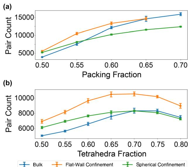
**Fig. 3** Number of tetrahedron-octahedron neighbor pairs at distances indicating the formation of the binary crystal—a proxy for crystallinity—(a) varying with packing fraction at the ideal stoichiometry and (b) varying with stoichiometry at  $\phi = 0.65$  packing fraction.
