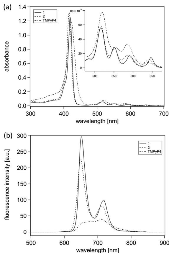
**Fig. 2** UV-vis (a) and fluorescence (b) spectra of porphyrins **1**, **2**, and **TMPyP4** (5 μM in 10 mM HEPES buffer (pH 7.4)). Fluorescence spectra were recorded with an excitation wavelength at 420 nm using a slit of 5 nm.
