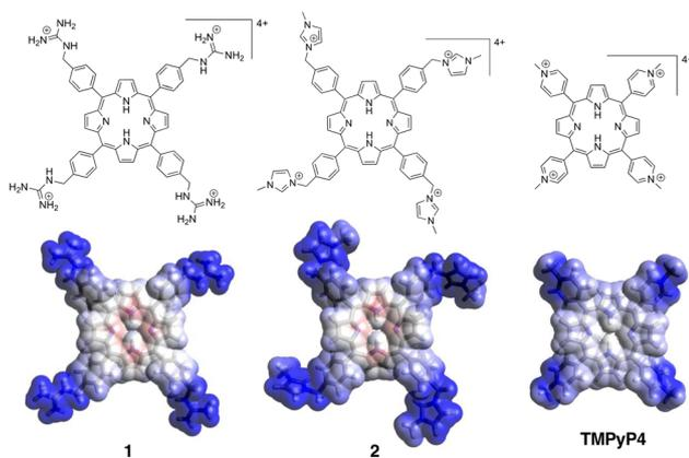
**Fig. 1** Chemical structures and electrostatic surface potential maps for porphyrin **1**, porphyrin **2**, and **TMPyP4**. Conformation optimization and electrostatic surface potential calculation were performed using the universal force field operated with Avogadro 1.2.0. Blue: lower electron density; red: higher electron density.
