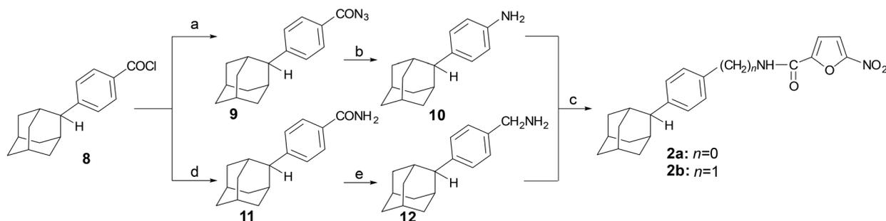
**Scheme 1** Reagents and conditions: a)  $\text{NaN}_3$ , acetone/water, 0 °C, 0.5 h, b) i. toluene, 95 °C, ii. HCl 36%, 95 °C, 1 h, 54% (from **8**) c) 5-nitro-2-furoic acid, HBTU, DIPEA, DCM/DMF 1:1 (v/v), RT, 24 h, 78% (**2a**), 70% (**2b**), d)  $\text{NH}_3$ , THF, 0 °C then RT, 0.5 h, 71%, e)  $\text{LiAlH}_4$ , THF, RT, 24 h, 66%.
