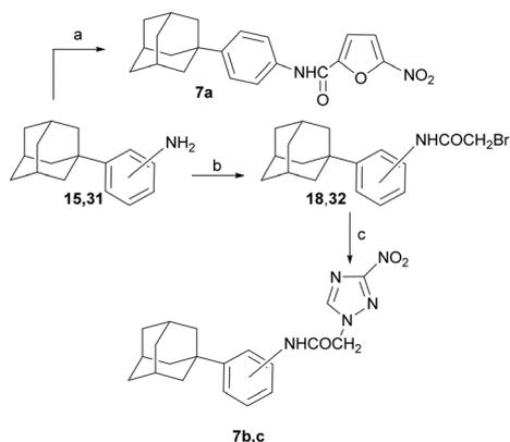
**Scheme 6** Reagents and conditions: a) 5-nitro-2-furoic acid, HBTU, DIPEA, DCM/DMF 1:1 (v/v), RT, 24 h, 76%; b) BrCH<sub>2</sub>COCl, Na<sub>2</sub>CO<sub>3</sub>, CHCl<sub>3</sub> - H<sub>2</sub>O, 0 °C to RT, 48 h, 84–89%; c) sodium 3-nitro-1,2,4-triazol-1-ide, DMF, 50 °C, 48 h, 52–91%.
