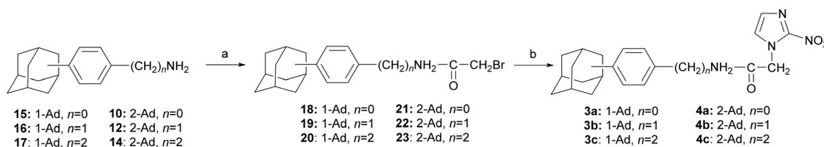
**Scheme 3** Reagents and conditions: a)  $\text{BrCH}_2\text{COCl}$ ,  $\text{Na}_2\text{CO}_3$ ,  $\text{CHCl}_3 - \text{H}_2\text{O}$ , 0 °C to RT, 48 h, b) sodium 2-nitroimidazol-1-ide, DMF, 80 °C, 48 h, 35% over two steps (**3a** from **15**), 38% (**3b** from **16**), 33% (**3c** from **17**), 23% (**4a** from **10**), 26% (**4b** from **12**), 31% (**4c** from **14**).
