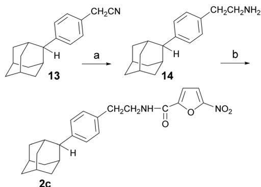
**Scheme 2** Reagents and conditions: a) BMS 2 M in toluene, THF, RT for 24 h then 50 °C for 5 h, 81%, b) 5-nitro-2-furoic acid, HBTU, DIPEA, DCM/DMF 1:1 (v/v), RT, 24 h, 76%.
