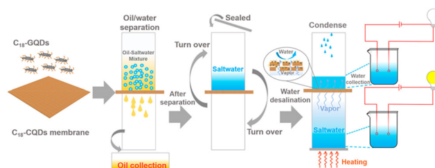
Fig. 10 Separation and saltwater desalination (reproduced with permission from ref. 116 ©, The American Chemical Society 2019). 116
