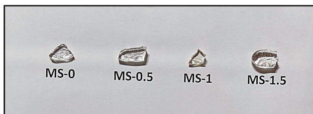
Fig. 1 Photograph of as-synthesized glass samples melted and annealed at 1550 °C and 400 °C, respectively.
