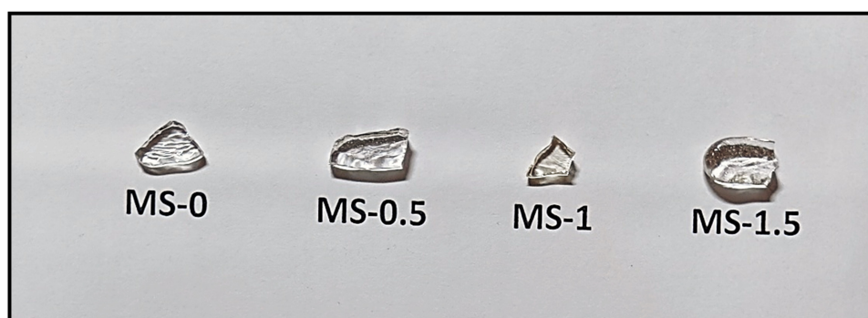
Figure 1: Photograph of as-synthesized glass samples melted and annealed at 1550^\circ\text{C} and 400^\circ\text{C} , respectively
