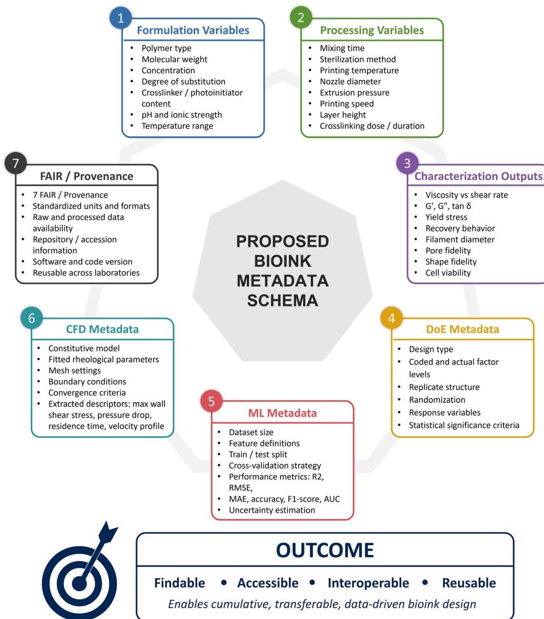
Fig. 7 Proposed bioink metadata schema for FAIR DoE–ML–CFD workflow.
