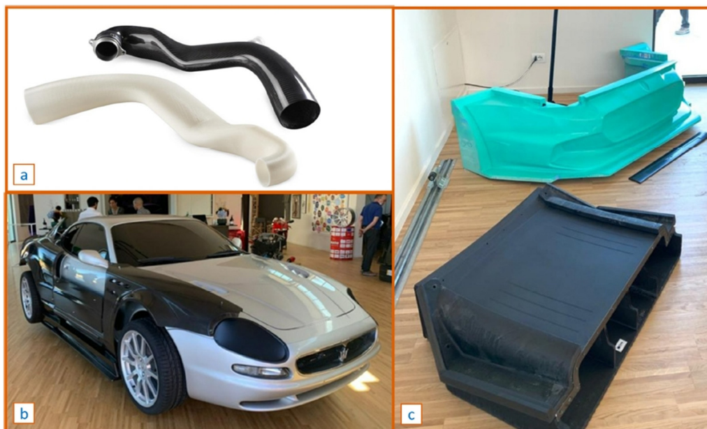
Fig. 28 Spare part reconstruction using CAM showing (a) inlet duct made of carbon fiber, (b) body components of Maserati MV 3200 GTC, and (c) related tooling, adapted from ref. 258 (open access).
