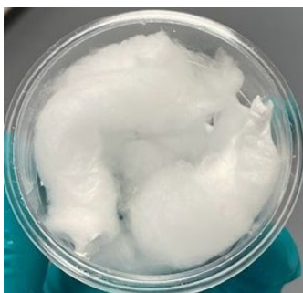
Figure 2. Optical image of a representative PGFs demonstrating the cotton-like morphology.
