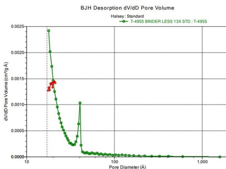
Fig. 8 BJH desorption pore size distribution ( dv/dD vs. pore diameter) of the synthesized sample calculated using Hasley standard model
