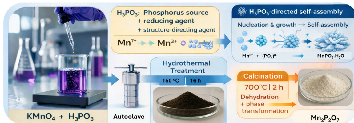
Fig. 1 Schematic illustration of the synthesis of \text{MnPO}_4 \cdot \text{H}_2\text{O} and \text{Mn}_2\text{P}_2\text{O}_7 .
