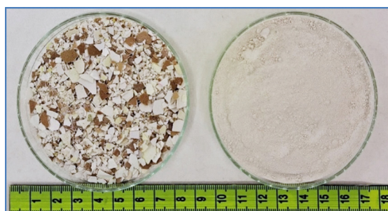
Fig. 2 Raw and mechanically processed eggshells.
