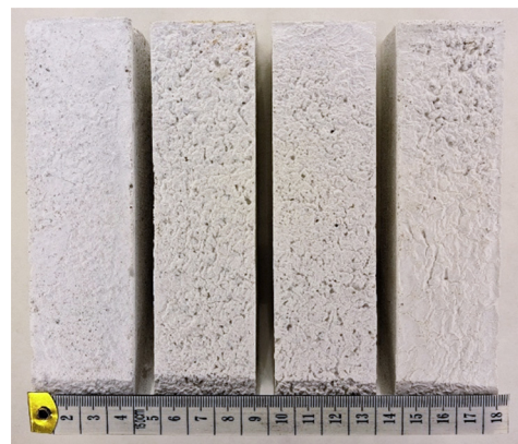
Fig. 3 Prismatic specimens of lime mortars, from left: LM-REF, LM-ES-25, LM-ES-50, LM-ES-75.
