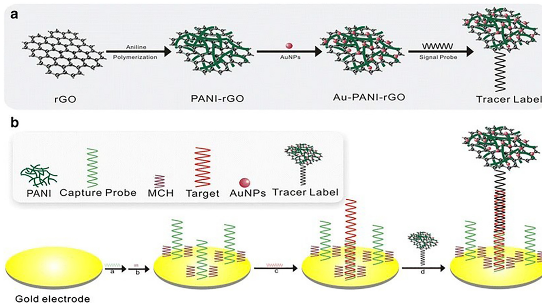
Fig. 13 Synthesis of the (a) Au-PANI-rGO, and (b) electrochemical DNA biosensor (reproduced with permission from ref. 87).
