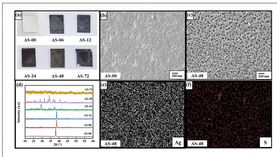
**Fig. 1** (a) Visual inspection of Ag films after sulfurization for 6, 12, 24, 48, and 72 hours, along with the untreated Ag reference. (b) SEM image of pristine Ag film. (c) SEM image of the  $Ag_2S$  film after 48 hours of sulfurization. (d) XRD patterns of Ag films (AS-00 to AS-72) corresponding to different sulfurization durations. (e) and (f) EDS elemental mapping of the 48-hour  $Ag_2S$  film showing the distribution of (e) Ag and (f) S.
