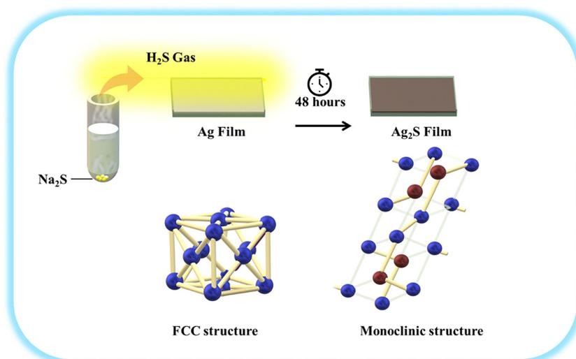
Scheme 2 Schematic representation of the structural changes from Ag to Ag<sub>2</sub>S.
