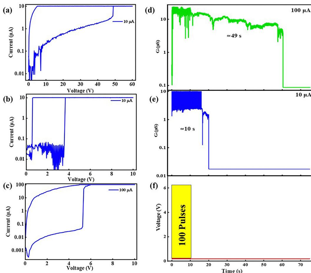
**Fig. 2** (a) 1st RS cycle at 10  $\mu$ A, RS graph at (b) 10  $\mu$ A and (c) 100  $\mu$ A. (d–f) Conductance potentiation and decay under 100  $\mu$ A (green) and 10  $\mu$ A (blue) current limits following pulsed stimulation.
