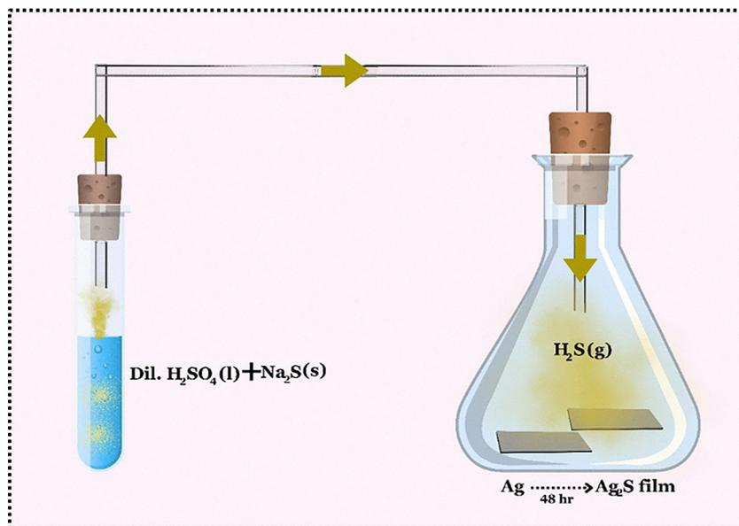
Scheme 1 Schematic diagram illustrating the passage of H<sub>2</sub>S gas over the Ag-deposited glass substrate.
