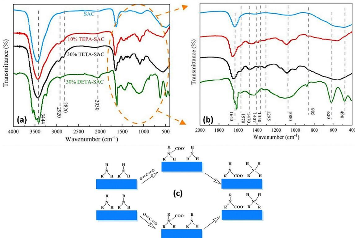
Fig. 10 (a) FT-IR spectra of various carbon materials; (b) magnified view of the region highlighted by the orange dashed circle; (c) schematic illustration of the potential CO<sub>2</sub> adsorption mechanisms on carbon surfaces functionalized with primary and secondary amine groups (reproduced from ref. 189 with permission from [Elsevier], copyright [2024]).
