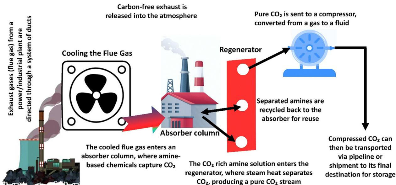
**Fig. 3** Schematic of amine-based post-combustion CO<sub>2</sub> capture, showing flue-gas cooling, CO<sub>2</sub> absorption in an amine scrubber, thermal regeneration of the solvent, amine recycling, and compression of purified CO<sub>2</sub> for transport and storage.
