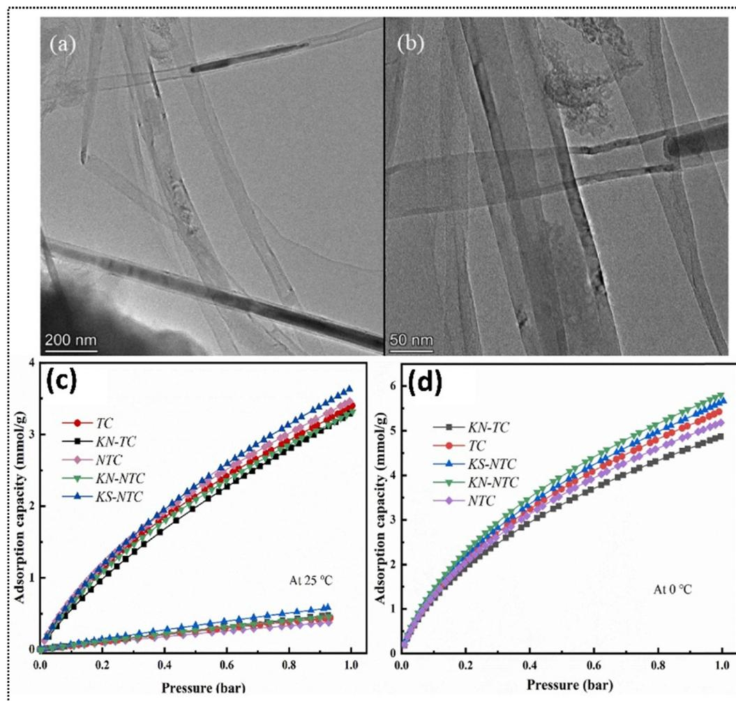
Fig. 14 (a and b) TEM images of the KS-NTC sample; (c) CO<sub>2</sub> and N<sub>2</sub> adsorption capacities of the carbon nanotube composite measured at 25 °C; (d) CO<sub>2</sub> and N<sub>2</sub> adsorption capacities at 0 °C (reproduced from ref. 215 with permission from [Elsevier], copyright [2024]).
