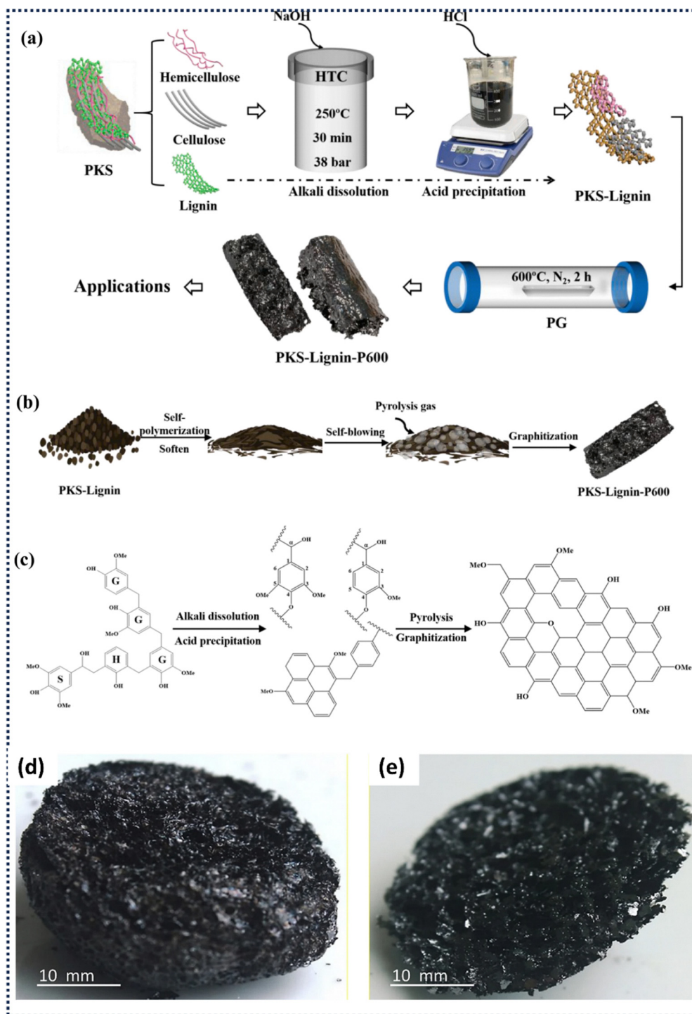
Fig. 16 (a) Schematic representation of the synthesis process for lignin-based carbon foam derived from palm kernel shells; (b and c) proposed reaction mechanism illustrating the key steps involved in the formation of the carbon foam structure (reproduced from ref. 242 with permission from [Elsevier], copyright [2022]); GO foams obtained employing the DTD and characterization methods, (d) 873.15 K (GO 9.00%), (e) 973.15 K (GO 5.25%) (reproduced from ref. 227 under the Creative Commons Attribution (CC BY) license).
