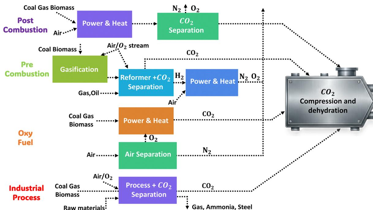
Fig. 5 Graphical representation of major  $\text{CO}_2$  capture routes with integrated energy and industrial systems before transport, storage, and utilization.
