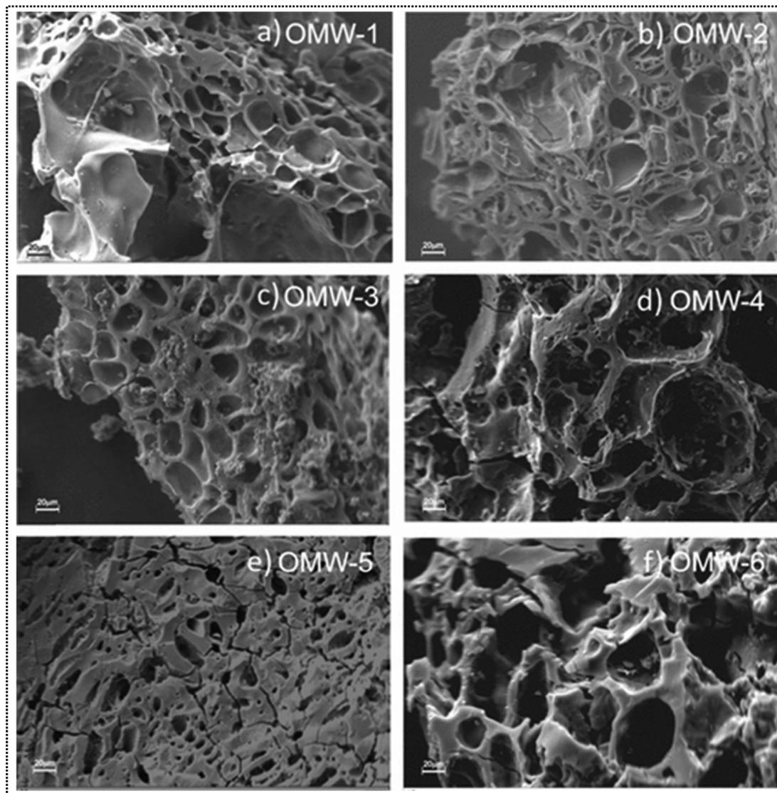
Fig. 9 SEM micrographs recorded at 1000 $\times$  magnification for the activated carbon samples: (a) OMW-1, (b) OMW-2, (c) OMW-3, (d) OMW-4, (e) OMW-5, and (f) OMW-6, illustrating the evolution of surface morphology under different activation conditions (reproduced from ref. 185 under the Creative Commons Attribution (CC BY 4.0) license).
