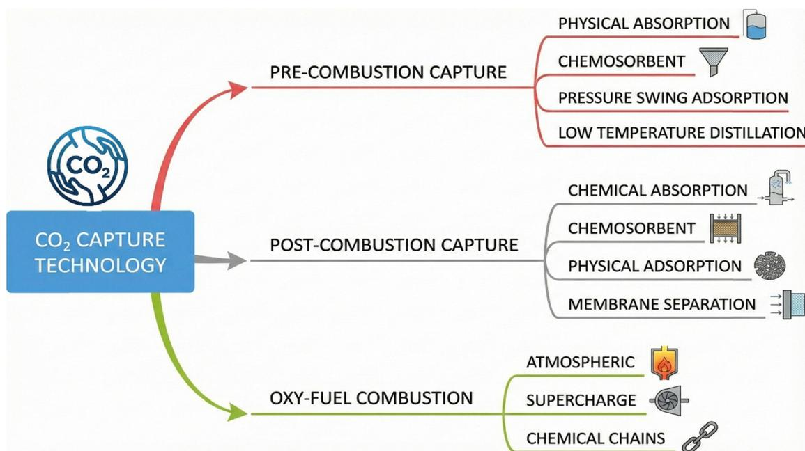
Fig. 4 CO<sub>2</sub> capture pathways and primary capture techniques in pre-combustion, post-combustion, and oxy-fuel processes.
