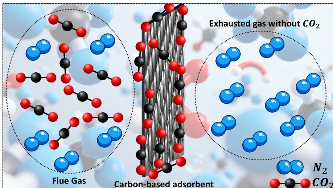
Fig. 7 Adsorption mechanism of CO<sub>2</sub> capture from flue gas *via* a carbon-based adsorbent.
