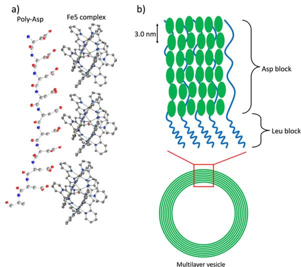
**Fig. 8** Hierarchical schematic illustration of the self-assembly of diblock copolypeptide amphiphiles **3/Fe5**, showing how diblock copolypeptide amphiphiles with Fe pentanuclear complexes (a) form a vesicular-like structure (b).
