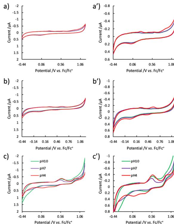
**Fig. 7** Cyclic voltammograms (CV) in 0.1 M NaClO<sub>4</sub> for hybrids of (a) **1/Fe5**, (b) **2/Fe5**, and (c) **3/Fe5**, prepared by the samples at different pH, where [Fe complex] = 0.1 mM. The sweep rate was 10 mV s<sup>-1</sup>. Panels (a')–(c') show enlarged views of the corresponding CVs in (a)–(c), respectively, with expanded current (vertical) axes to highlight electrochemical features.
