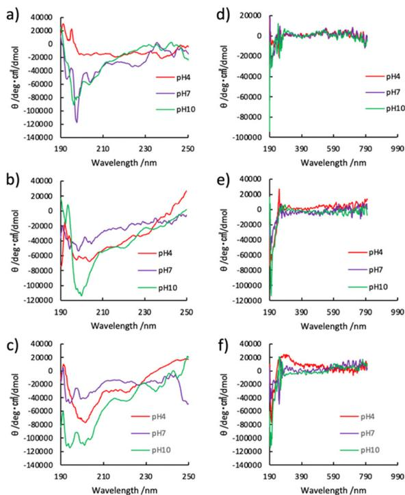
**Fig. 6** CD spectra for hybrid of (a) **1/Fe5**, (b) **2/Fe5**, and (c) **3/Fe5**, prepared by the samples at different pH, where [Fe complex] = 0.1 mM. CD spectra over a broader range (190–900 nm), (d) **1/Fe5**, (e) **2/Fe5**, and (f) **3/Fe5** show a slight induced circular dichroism (ICD) around 500 nm for **2/Fe5** and **3/Fe5** at pH 4.
