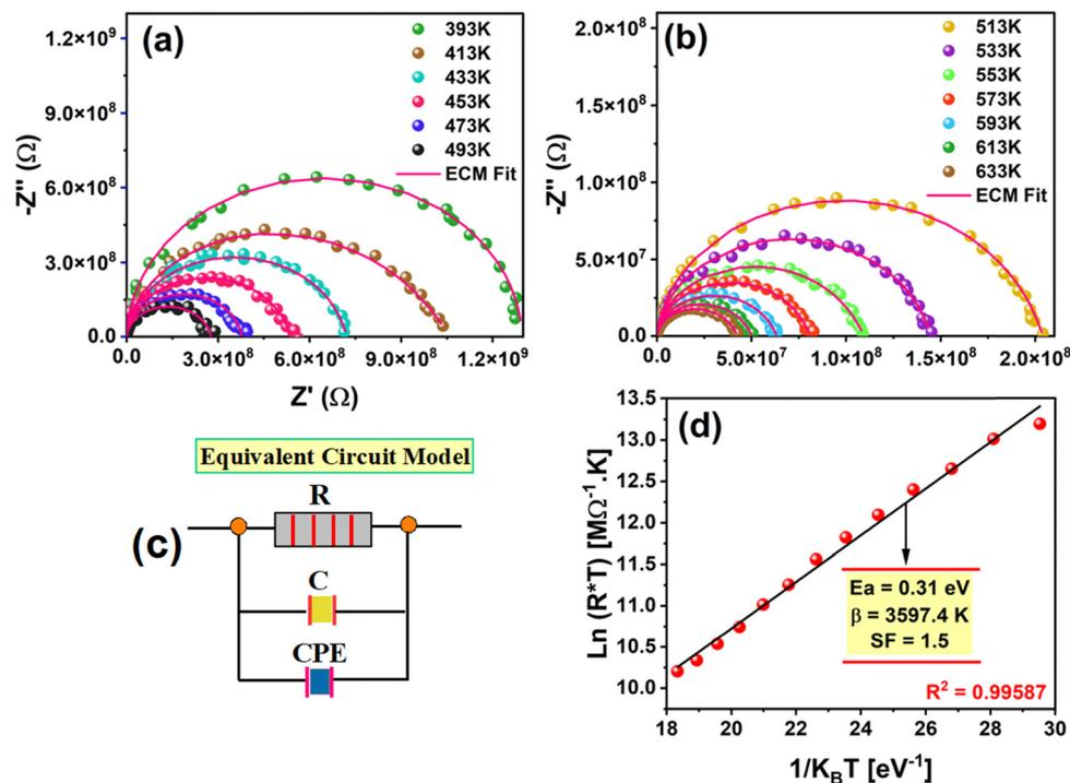
Fig. 10 (a) and (b) Nyquist plots ( $Z''$  vs.  $Z'$ ) of the NCPO compound recorded at various temperatures; (c) equivalent circuit model used for impedance fitting; (d) Arrhenius plot of  $\ln(R \times T)$  as a function of inverse temperature ( $1000/T$ ), illustrating thermally activated conduction behavior.
