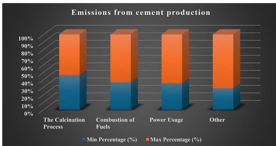
Fig. 1 Schematic breakdown of the primary sources of CO<sub>2</sub> emissions in conventional Portland cement manufacturing. Process emissions from the calcination of limestone are the largest contributor, followed by emissions from the combustion of fossil fuels required to heat the kiln.<sup>2,20,21</sup>
