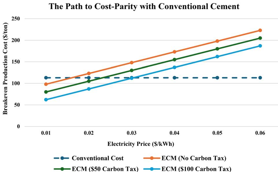
Fig. 25 Breakeven production cost for the electrochemical HOR pathway as a function of electricity price, evaluated under three carbon tax scenarios (\$0, \$50, and 100 per ton of  $\text{CO}_2$ ). The horizontal dashed line represents the benchmark cost of conventional cement.<sup>21,30</sup>
