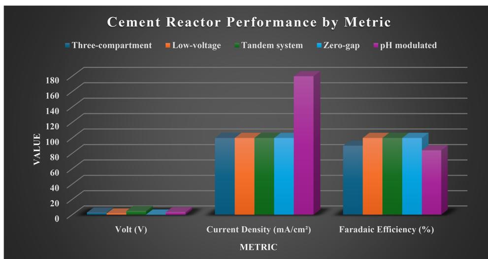
Fig. 20 Performance comparison of different electrochemical cement reactor designs across three key metrics: cell voltage, current density, and Faradaic efficiency (FE).
