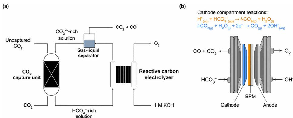
Fig. 30 (a) Integrated system for CO<sub>2</sub> capture and utilization: alkaline absorption of CO<sub>2</sub> produces a liquid eluent for direct transfer to the electrolyzer. (b) Reactive carbon electrolyzer cathode compartment shows i-CO<sub>2</sub> liberation via BPM and subsequent reduction to CO<sub>2</sub>. Anode compartment fed with 1 M KOH. Reprinted with permission from ref. 59. Copyright (2024) the Royal Society of Chemistry.
