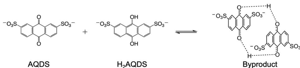
Fig. 16 Chemical structures of the AQDS/H<sub>2</sub>AQ redox mediator and the quinone dimer byproduct formed at the anode. Reprinted with permission from ref. 27. Copyright (2025) American Chemical Society.
