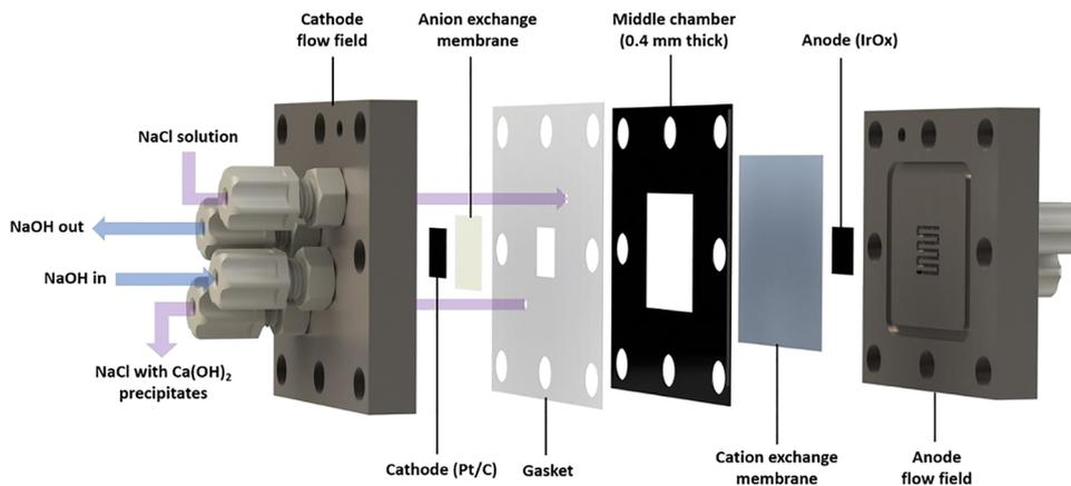
Fig. 13 Expanded view of the electrolyzer assembly employed for the anion-mediated ECE process depicted in Fig. 12. The diagram details the arrangement of the specific components, including the IrO<sub>2</sub> anode, Pt/C cathode, and the dual-membrane stack (CEM and AEM). Reprinted with permission from ref. 32. Copyright (2023) American Chemical Society.
