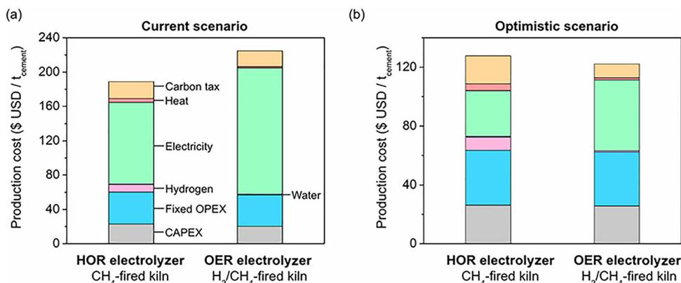
Fig. 24 Techno-economic comparison of electrochemical cement production using HOR and OER electrolyzers. The costs, broken down by CAPEX and OPEX components, are evaluated under two distinct scenarios: (a) a Current Market Scenario reflecting existing energy/carbon economics and (b) an Optimistic Future Projection based on low-cost solar power and stringent climate policy. Reprinted with permission from ref. 30. Copyright (2023) American Chemical Society.
