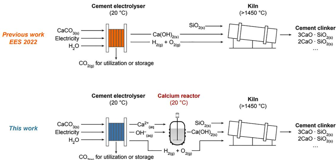
**Fig. 11** Comparison of electrochemical cement production pathways. Top: direct *in situ*  $\text{Ca}(\text{OH})_2$  synthesis within the electrolyzer. Bottom: tandem approach decoupling electrochemical ion generation from *ex situ* precipitation in a separate reactor. Both routes produce  $\text{Ca}(\text{OH})_2$  precursors for subsequent clinker formation. Reprinted with permission from ref. 26. Copyright (2025) the Royal Society of Chemistry.
