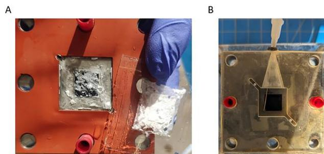
Fig. 19 This figure demonstrates a mechanical strategy to counteract the accumulation of Ca(OH)<sub>2</sub> precipitate (A) observed during stability tests. The solution is a custom flow field with an integrated wiper (B) designed for *in operando* cleaning of the electrolyzer. Reprinted with permission from ref. 32. Copyright (2023) American Chemical Society.
