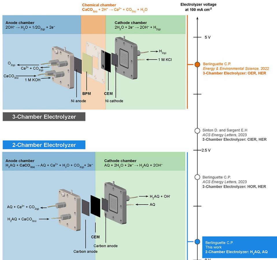
Fig. 15 Operating voltage comparison at 100 mA cm<sup>-2</sup> for 3-chamber and 2-chamber cement electrolyzers. A schematic illustrates reactor configurations and key electrochemical reactions: hydrogen oxidation (HOR), chloride oxidation (CIER), hydrogen evolution (HER), and oxygen evolution (OER). Reprinted with permission from ref. 27. Copyright (2025) American Chemical Society.
