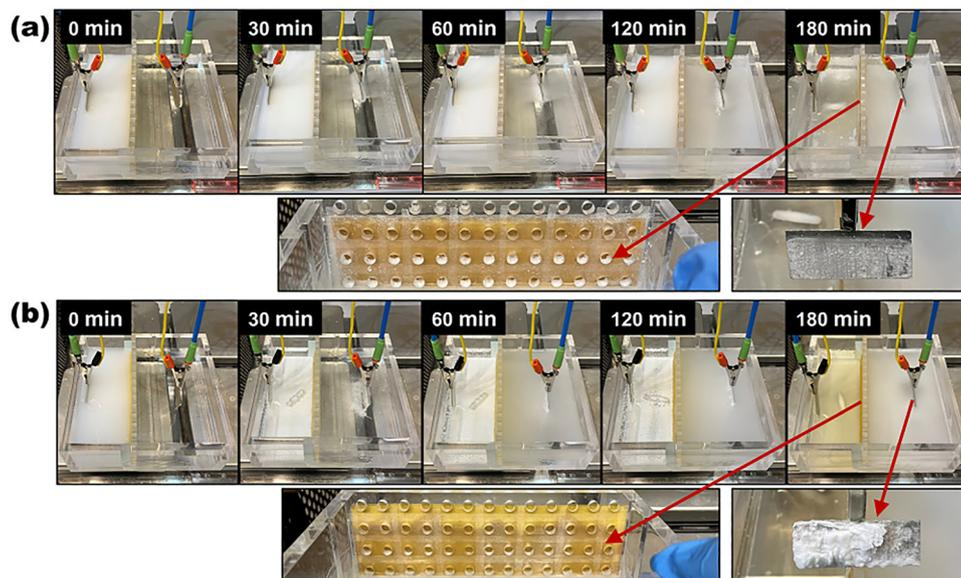
Fig. 6 A sequence of images captured over time shows the formation of  $\text{Ca}(\text{OH})_2$  during the electrolysis process within a cement clinker precursor reactor. The deposition patterns of the  $\text{Ca}(\text{OH})_2$  product on the electrode and membrane are displayed after 3 hours for two different catholyte conditions: (a) an initial catholyte with no calcium ions and (b) one containing  $0.2 \text{ M Ca}^{2+}$ .
