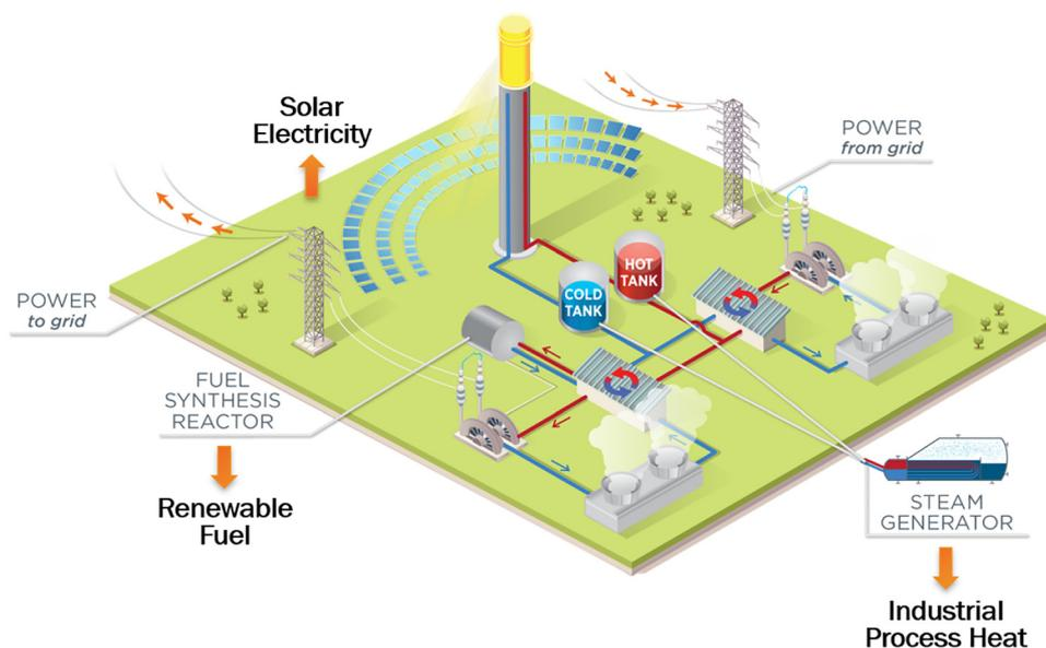
Fig. 31 U.S. Department of Energy schematic outlining diverse pathways for the integration of concentrated solar power into broad industrial applications.<sup>2,74</sup>
