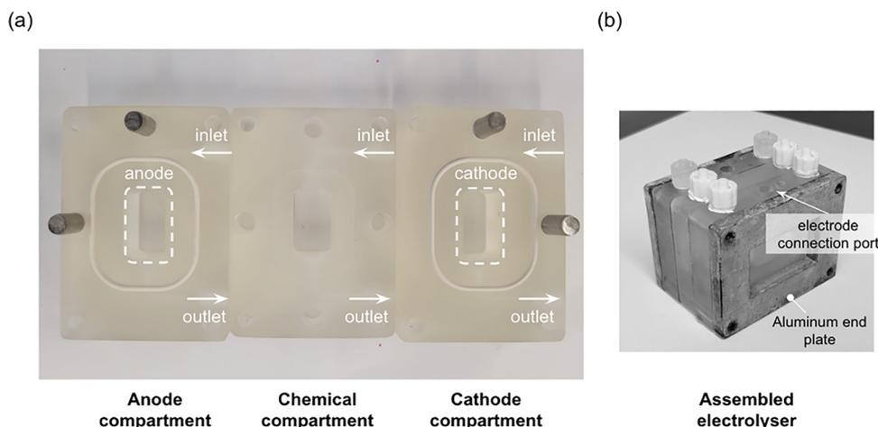
**Fig. 10** Images of an additively manufactured three-chamber electrolyzer for cement production. (a) Exploded view showing the separate anode, chemical reaction, and cathode chambers. (b) The fully assembled cell secured with aluminum compression plates. Reprinted with permission from ref. 30. Copyright (2023) American Chemical Society.
