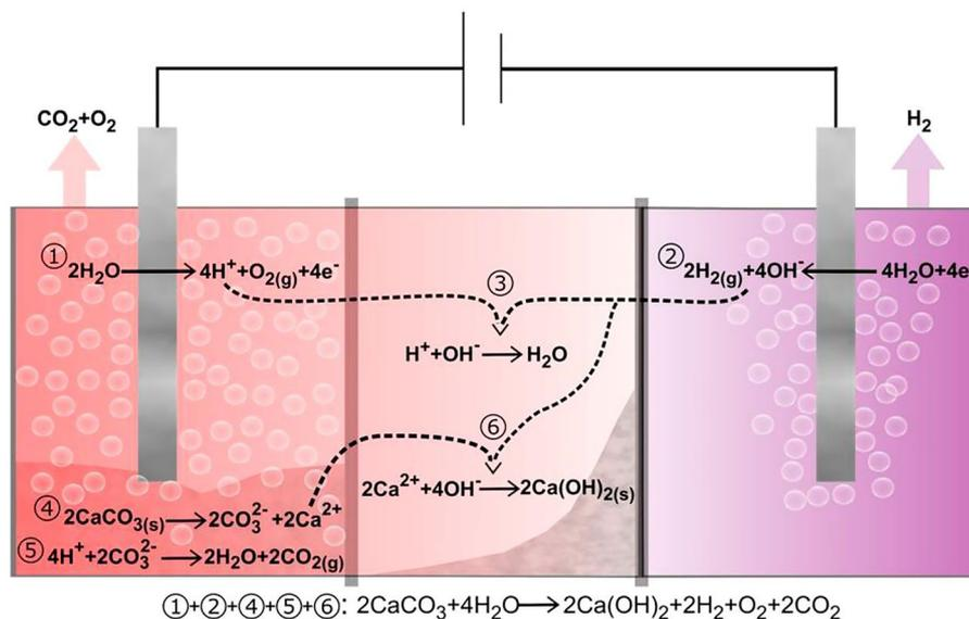
Fig. 3 The fundamental principle of electrochemical cement synthesis. Water electrolysis generates a pH gradient, with protons ( $\text{H}^+$ ) dissolving limestone ( $\text{CaCO}_3$ ) at the anode and hydroxide ions ( $\text{OH}^-$ ) precipitating calcium hydroxide ( $\text{Ca}(\text{OH})_2$ ) at the cathode. Hydrogen, oxygen, and pure  $\text{CO}_2$  are generated as valuable co-products.<sup>24</sup>
