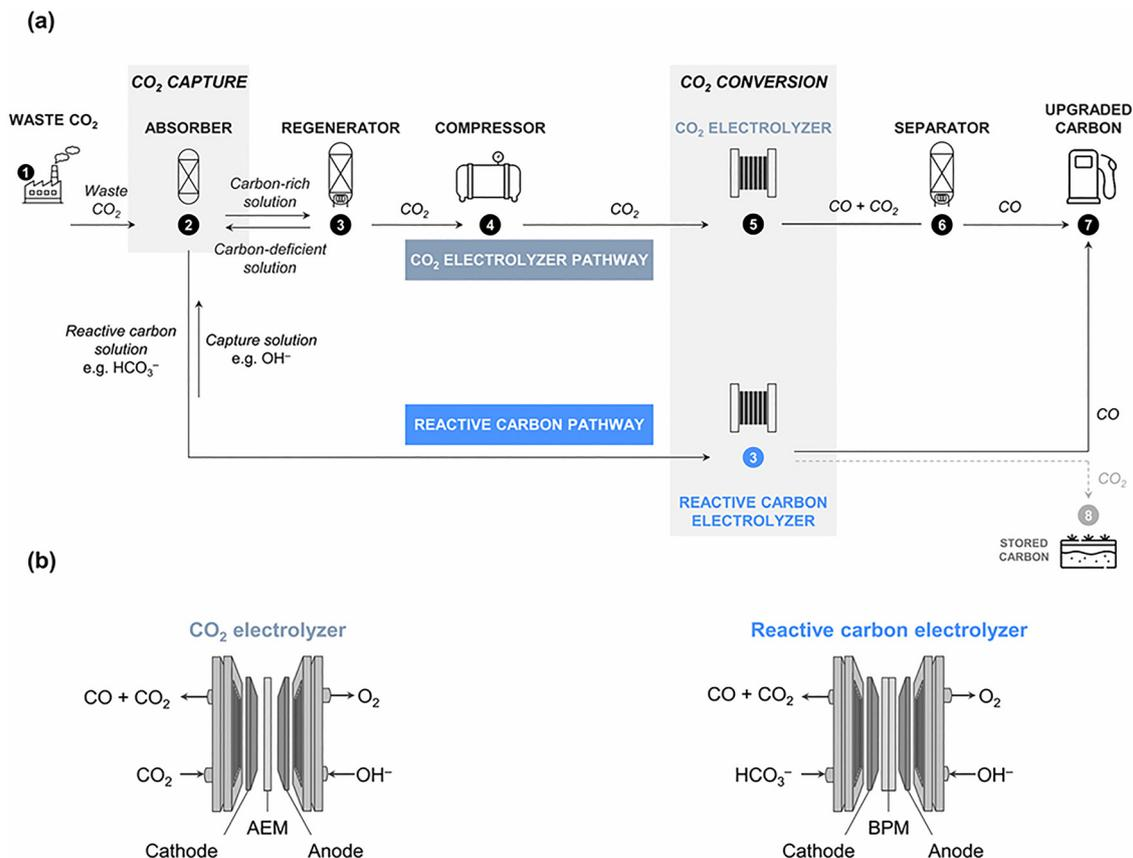
Fig. 29 (a) Comparison of CO<sub>2</sub> capture and utilization strategies. While both use alkaline absorption, the CO<sub>2</sub> electrolyzer requires thermal/vacuum regeneration to release gas, whereas the reactive carbon electrolyzer processes the liquid directly, avoiding gas liberation steps. (b) Cross-sectional view of electrolyzer components, including BPM and AEM. Reprinted with permission from ref. 59. Copyright (2024) the Royal Society of Chemistry.
