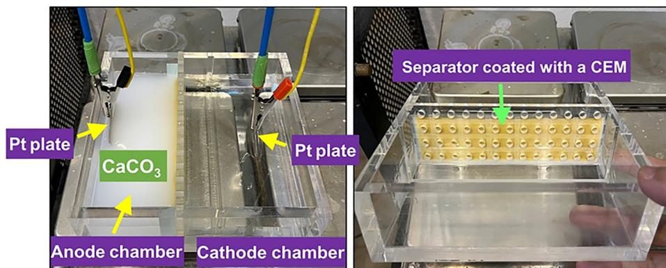
Fig. 5 Image depicting an H-cell electrolyzer (14 cm<sup>3</sup>) configured for the electrochemical synthesis of cement clinker precursors.<sup>29</sup>
