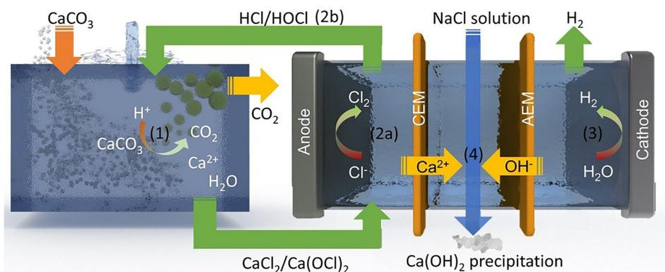
**Fig. 12** A diagram of the electrochemical calcium extraction (ECE) method for producing calcium hydroxide ( $\text{Ca}(\text{OH})_2$ ). Reprinted with permission from ref. 32. Copyright (2023) American Chemical Society.
