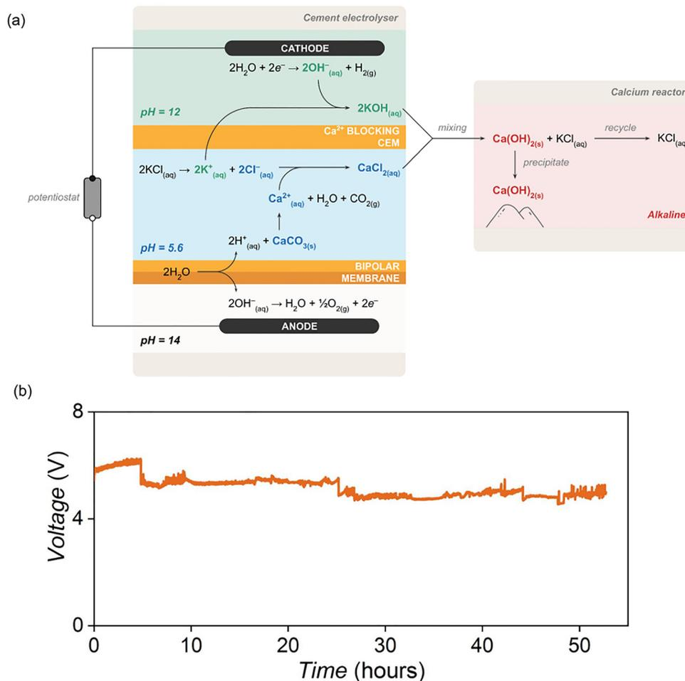
Fig. 18 Fouling mitigation *via* orthogonalized ion vectors. (a) Schematic of the composite PANI-CEM selectively blocking Ca<sup>2+</sup> to decouple precipitation from electrolysis. (b) Voltage stability over 50 hours at 100 mA cm<sup>-2</sup>, demonstrating the elimination of fouling-induced degradation. Reprinted with permission from ref. 26. Copyright (2025) the Royal Society of Chemistry.
