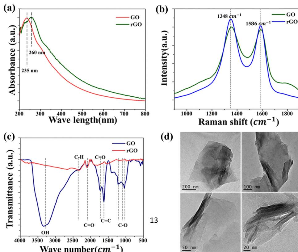
Fig. 2 Characterization of GO and rGO nanosheets. (a) UV-Vis spectra with maximum absorbance of GO at  $235\text{ nm}$  and that of rGO at  $260\text{ nm}$ . (b) Raman spectra with the corresponding D band at  $1348\text{ cm}^{-1}$  and G band at  $1586\text{ cm}^{-1}$ . (c) Fourier-transform infrared (FTIR) spectra with C–H, C=O, C=C, C–O, and O–H stretching. (d) Transmission electron microscopy (TEM) images of rGO nanosheets with a thickness of few to several layers.
