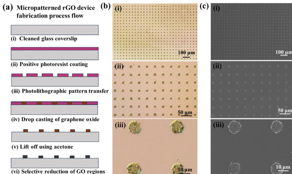
**Fig. 3** The micro-patterned rGO device with an array of 10  $\mu\text{m}$ -diameter rGO islands and an inter-island spacing of 30  $\mu\text{m}$  fabricated on a glass coverslip. (a) Illustration of the process steps (i)–(vi) involved in fabricating the micropatterned rGO device. (b) Optical images of the rGO device (i)–(iii) at different magnifications and (c) SEM images of the micro-patterned rGO device (i)–(iii) at different magnifications, revealing the surface morphology of the device.
