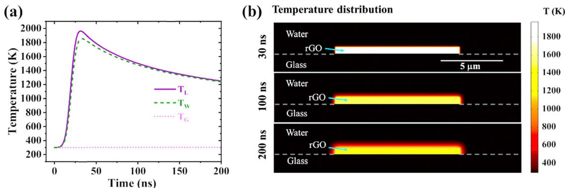
Fig. 5 Simulation results using COMSOL Multiphysics at a fluence of  $28 \text{ mJ cm}^{-2}$ . (a) Temporal evaluation of rGO, water, and glass substrate temperatures at an arbitrary point at the interface. (b) Spatial temperature distribution at 30 ns, 100 ns, and 200 ns showing thermal transport from the hot rGO lattice microstructure to the adjacent water.
