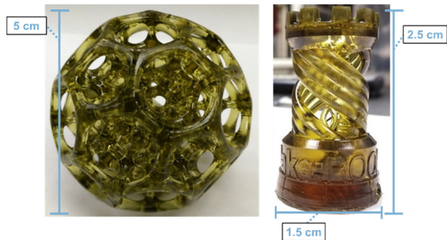
Fig. 6 Examples of objects printed using resin formulation consisting of monomer 4 , Ru-2 , CPTX, bTBTT, DMAP, Irganox ® 1076, and Irgafos ® 168.
