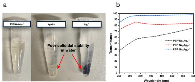
Fig. 6 Photographs of the PEP-Na<sub>5</sub>Ag<sub>1</sub>-l, AgNPs, and Ag<sub>2</sub>O (a). Transmittance (%T) spectra of the PEP-Na<sub>1</sub>Ag<sub>1</sub>-l, PEP-Na<sub>2</sub>Ag<sub>1</sub>-l, and PEP-Na<sub>5</sub>Ag<sub>1</sub>-l (b).
