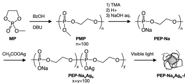
Fig. 1 Synthesis of PEP·Na<sub>x</sub>Ag<sub>y</sub>-l.
