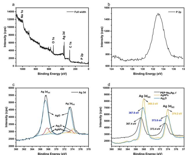
Fig. 5 X-ray photoelectron spectroscopy full spectrum (a), P<sub>2p</sub> (b), Ag<sub>3d</sub> (c). The Ag<sub>3d</sub> comparison of the PEP-Na<sub>5</sub>Ag<sub>1</sub>-l, AgNPs, and Ag<sub>2</sub>O (d).
