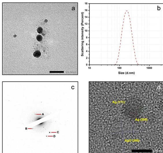
Fig. 4 Transmission electron microscopy images (a), dynamic light scattering measurement (b), selected area electron diffraction patterns (c), and high-resolution TEM images (d) of PEP-Na<sub>5</sub>Ag<sub>1</sub>-l.
