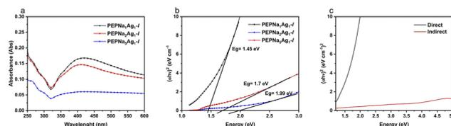
Fig. 3 UV-Vis spectra (a) and Tauc plot (b) of the  $\text{PEP}\cdot\text{Na}_1\text{Ag}_1$ -l,  $\text{PEP}\cdot\text{Na}_2\text{Ag}_1$ -l, and  $\text{PEP}\cdot\text{Na}_5\text{Ag}_1$ -l nanocomposites. Direct and indirect band gap of the  $\text{PEP}\cdot\text{Na}_1\text{Ag}_1$ -l (c).
