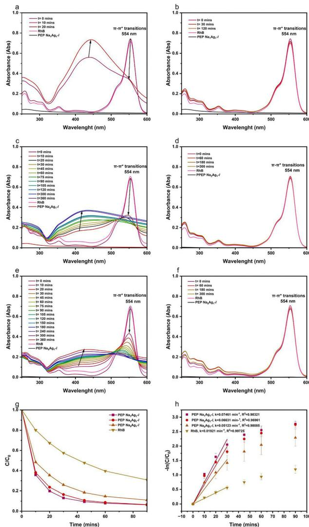
Fig. 7 UV-Vis spectra showing RhB degradation by PEP-Na<sub>1</sub>Ag<sub>1</sub>-l (a), (b), PEP-Na<sub>2</sub>Ag<sub>1</sub>-l (c), (d), and PEP-Na<sub>5</sub>Ag<sub>1</sub>-l (e), (f) under visible light and dark conditions, respectively. The  $C/C_0$  ratio (g), and first-order kinetics of PEP-Na<sub>1</sub>Ag<sub>1</sub>-l, PEP-Na<sub>2</sub>Ag<sub>1</sub>-l, PEP-Na<sub>5</sub>Ag<sub>1</sub>-l, and the control sample are also shown (h).
