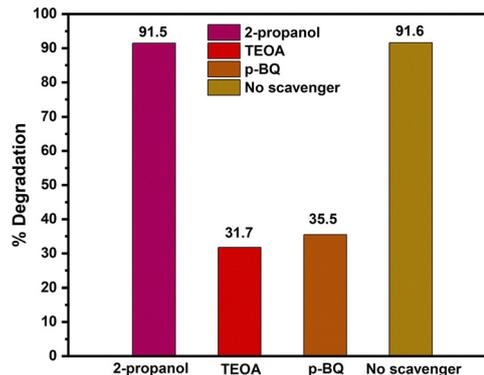
Fig. 9 Free radical scavenger test of PEP-Na<sub>5</sub>Ag<sub>1</sub>-I. The h<sup>+</sup>, OH<sup>•</sup>, and O<sub>2</sub><sup>•−</sup> radicals were removed using triethanolamine (TEOA), 2-propanol, and *p*-benzoquinone (*p*-BQ), respectively. The control sample did not have any scavengers.
