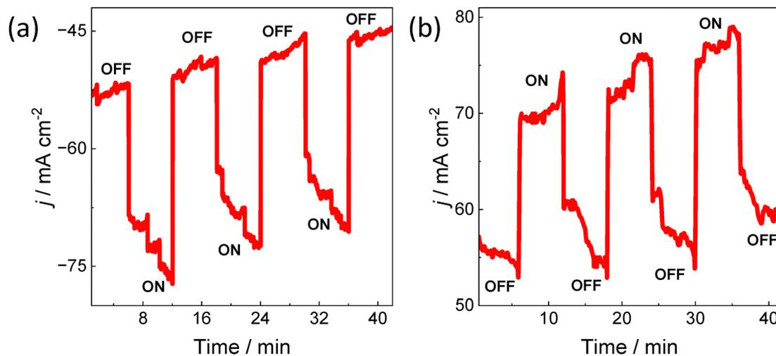
Fig. 11 Transient photocurrent response of the NiCoP/ $g\text{-C}_3\text{N}_4$  electrode under chopped visible-light illumination recorded at (a) cathodic potential, and (b) anodic potential.
