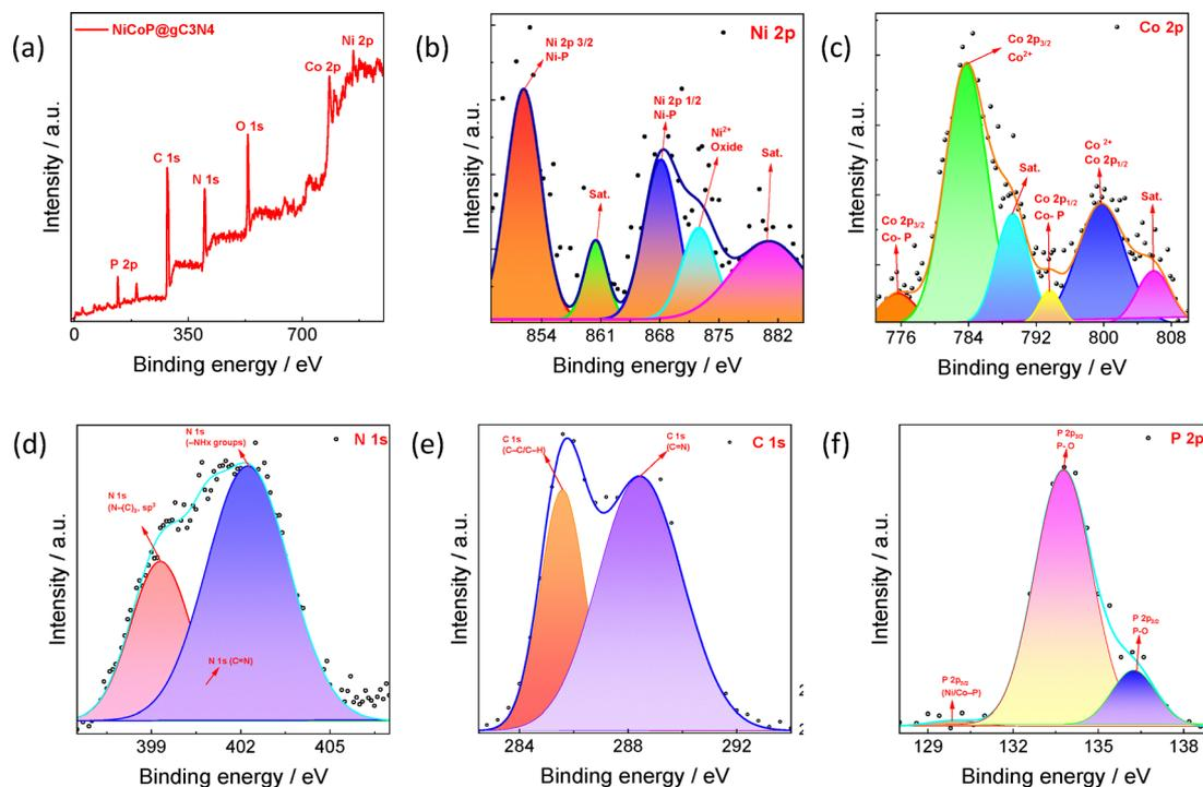
Fig. 5 XPS spectra of NiCoP/g-C<sub>3</sub>N<sub>4</sub>: (a) survey spectra of NiCoP/g-C<sub>3</sub>N<sub>4</sub>, (b) Ni 2p, (c) Co 2p, (d) N 1s, (e) C 1s, and (f) P 2p.
