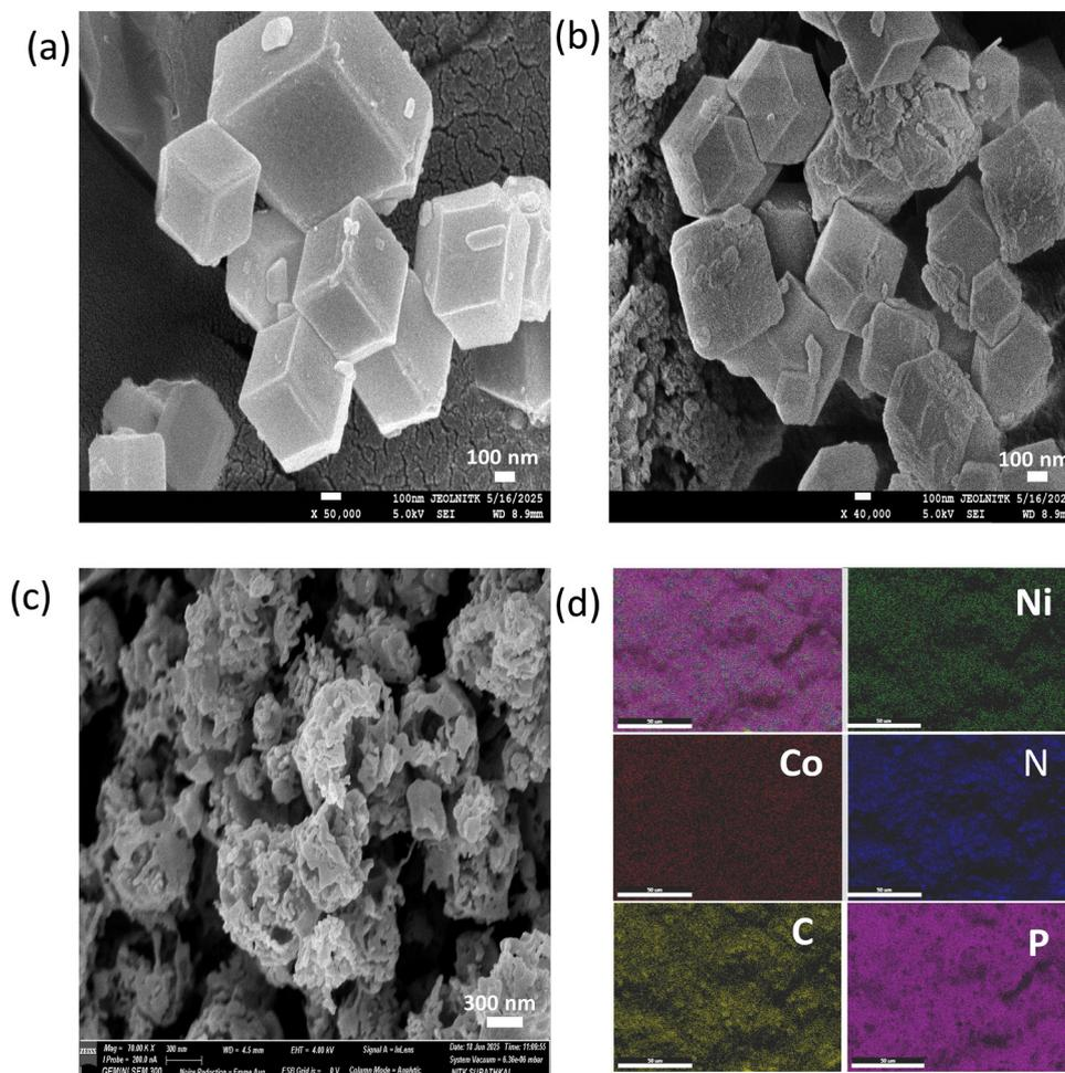
Fig. 3 FESEM of (a)  $\text{NiCo-MOF}$ , (b)  $\text{NiCo-MOF}/g\text{-C}_3\text{N}_4$ , (c)  $\text{NiCoP}/g\text{-C}_3\text{N}_4$ , and (d) colour mapping of  $\text{NiCoP}/g\text{-C}_3\text{N}_4$ , and corresponding elemental mapping (Ni, Co, N, C, P).
