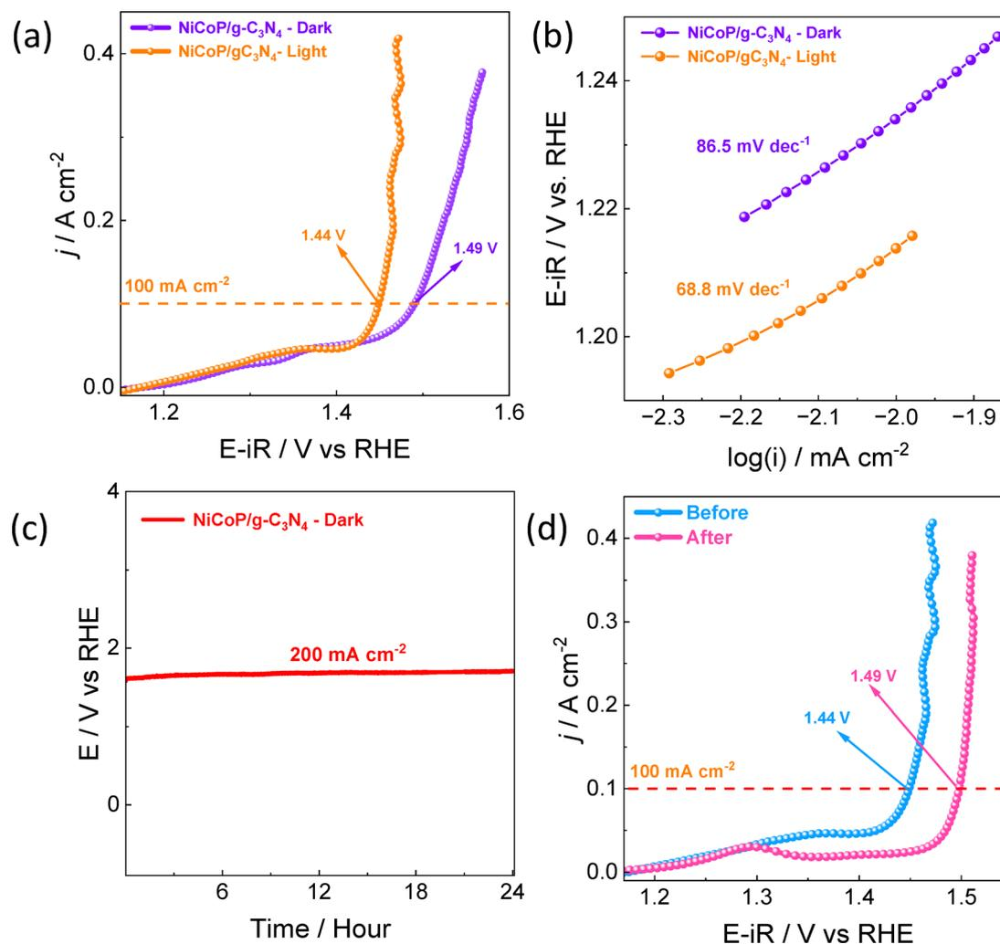
Fig. 10 (a)  $iR$  corrected LSV of NiCoP/ $g\text{-C}_3\text{N}_4$  in dark and illuminated conditions, (b) Tafel plot of NiCoP/ $g\text{-C}_3\text{N}_4$  in dark and illuminated conditions, (c) 24 hours of chronopotentiometry test for NiCoP/ $g\text{-C}_3\text{N}_4$  under illuminated conditions at a current density of  $-200\text{ mA cm}^{-2}$ , and (d)  $iR$  corrected LSV of NiCoP/ $g\text{-C}_3\text{N}_4$  in illuminated conditions before and after the chronopotentiometry test.
