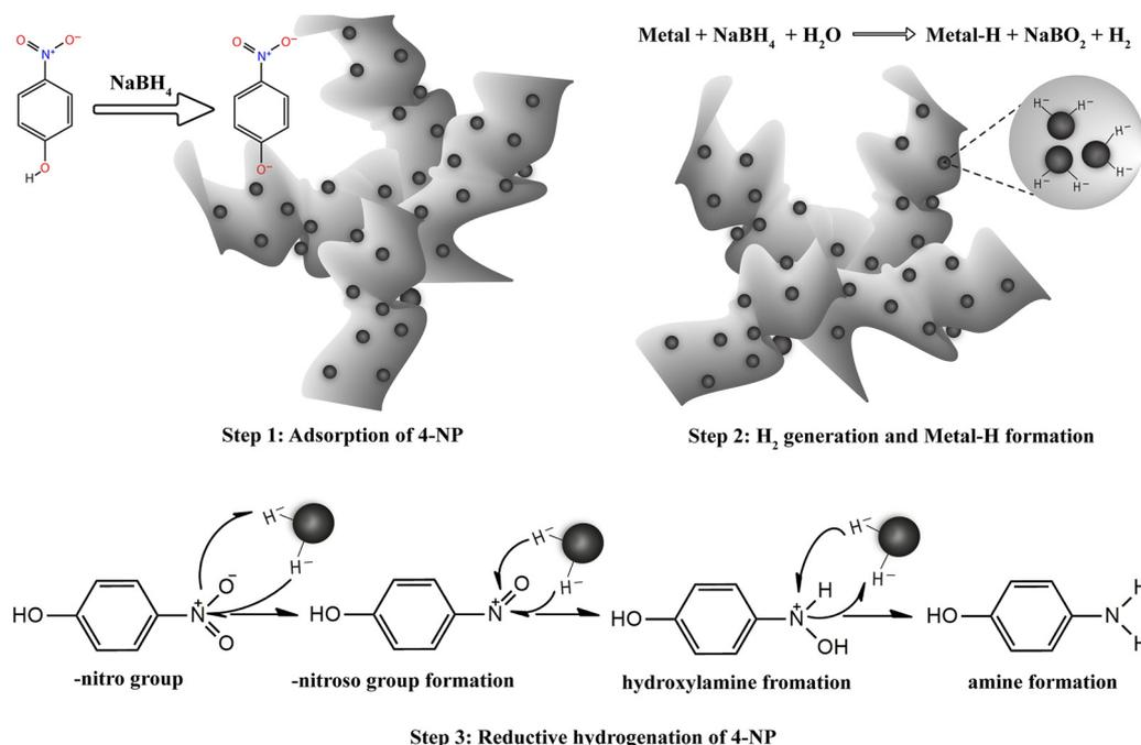
Fig. 7 A possible mechanism for the reduction of 4-NP catalyzed by the Ni-reline.
