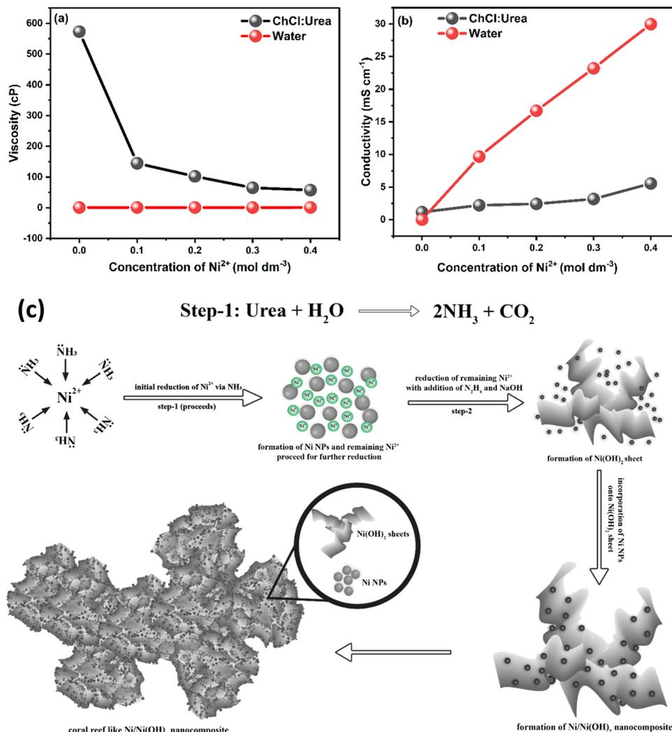
Fig. 4 Effect of Ni<sup>2+</sup> concentration on (a) viscosity, (b) conductivity of aqueous and reline systems and (c) schematic illustration of the Ni/Ni(OH)<sub>2</sub> formation in reline system.
