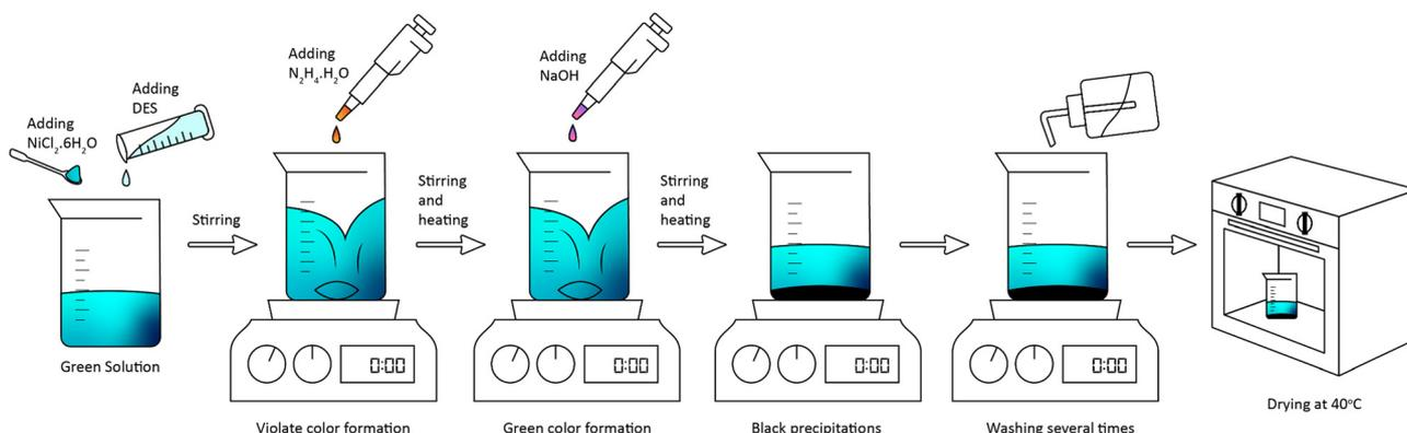
Fig. 1 Schematic representation of the synthesis of Ni-reline.
