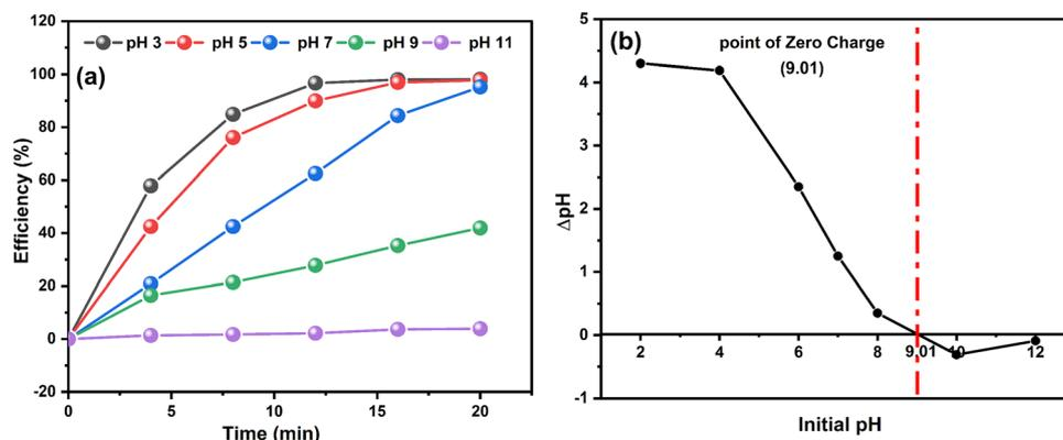
Fig. 6 (a) Effect of solution's pH in catalytic hydrogenation reaction of 4-NP (b) Determination of isoelectric point of Ni-reline (the reaction conditions included, 4-NP concentration: 1 mM;  $\text{NaBH}_4$  concentration: 10 mM; catalyst dosage: 5 mg; temperature: 25 °C).
