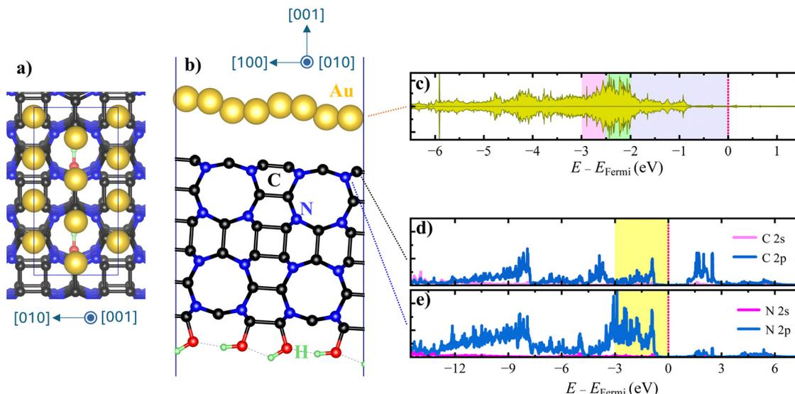
**Fig. 1** (a) and (b) Top and side views of the optimised structure of the single-layer Au nanosheet supported on C<sub>3</sub>N<sub>2</sub>. (c) The partial Au 5d density of states; the DOS outside the presented energy range is negligible. (d) and (e) The partial 2s and 2p DOS of the interface C and N, respectively.
