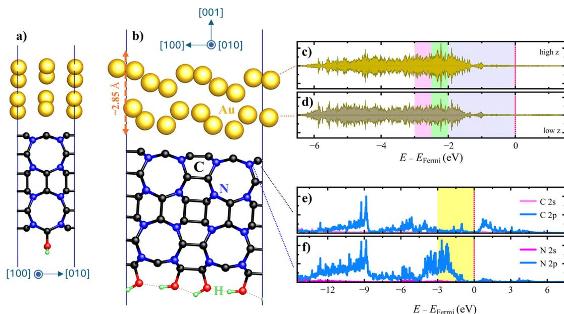
**Fig. 2** (a) and (b) Different side views of the optimised structure of the Au nanosheet supported on C<sub>3</sub>N<sub>2</sub>. (c) and (d) The partial Au 5d density of states resolved by layers. Au 5d DOS outside the presented energy range is negligible. (e) and (f) The partial 2s and 2p DOS of the interface C and N, respectively.  $z$  denotes the Au atoms' fractional coordinates along the long edge.
