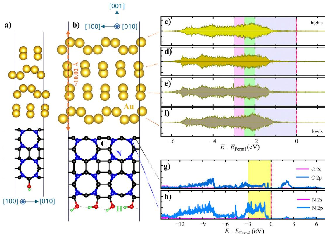
Fig. 3 (a) and (b) Different side views of the optimised four-layer Au<sub>x</sub>@C<sub>3</sub>N<sub>2</sub> interface. (c) through (f) The partial Au 5d density of states resolved by layers. (g) and (h) The partial 2s and 2p DOS of the interface C and N, respectively. *z* denotes the Au atoms' fractional coordinates along the long edge [001].
