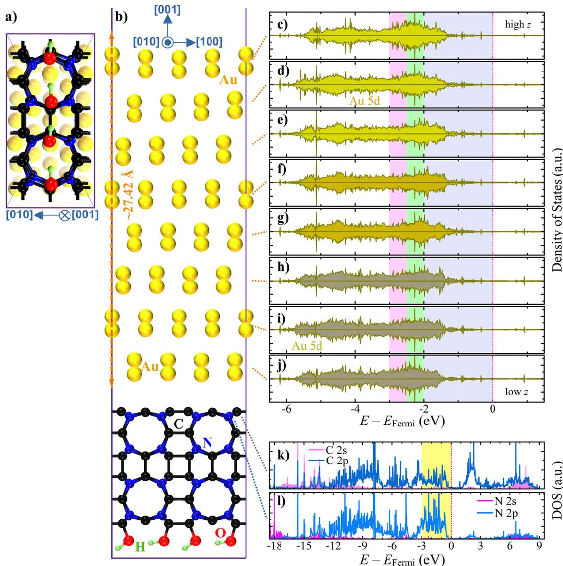
Fig. 4 (a) and (b) Top and side view of the optimised structure of the Au nanosheet supported on  $C_3N_2$ . (c) through (j) The partial Au 5d density of states resolved by layers. Au 5d DOS outside the presented energy range is negligible. (k) and (l) The partial 2s and 2p DOS pertaining to the interface C and N, respectively.  $z$  denotes the Au atoms' fractional coordinates along the long edge.
