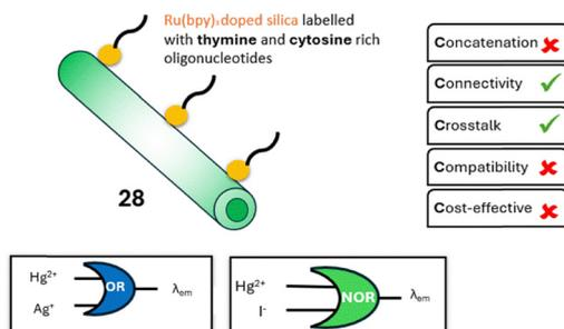
Fig. 32 Multiwalled carbon nanotube (MCNT) with Ru(bpy)<sub>3</sub> silica and thymine and cytosine oligonucleotide functionalisation.<sup>88</sup>
