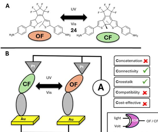
Fig. 23 Photonic memristor **24**, the diarylethene unit can photonically switch between open form (OF) and closed form (CF).<sup>65</sup>
