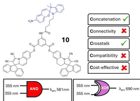
Fig. 8 Molecular logic gate **10** as a fully photonic AND and XOR gate functions.<sup>33</sup>
