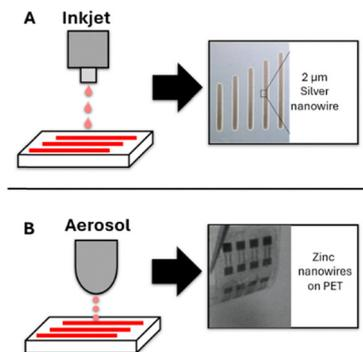
Fig. 30 3D printing of nanowires, images reproduced from ref. 78 and 79 with permission from ACS, copyright 2015, and RSC, copyright 2013 respectively.
