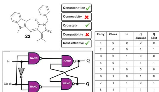
Fig. 21 Fully photonic molecular memory unit **22**.<sup>60</sup>
