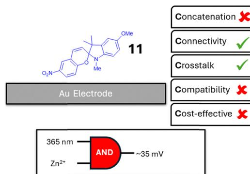
Fig. 9 Molecular logic gate **11** bound to a gold electrode.<sup>34</sup>
