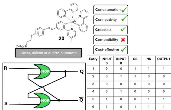
Fig. 18 Molecular logic gate **20** as a substrate-bound SR latch.<sup>57</sup>
