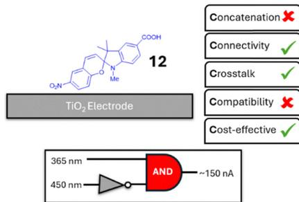
Fig. 10 Molecular logic gate **12**.<sup>35</sup>
