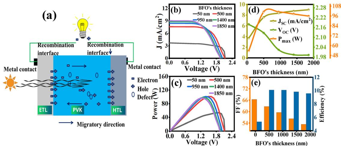
Fig. 3 (a) Schematic of the effect of the absorbing layer's thickness on the performance of the solar cell, (b)  $J$ - $V$  curve and (c)  $P$ - $V$  curve of the  $\text{TiO}_2/\text{BFO}/\text{Spiro-O-MeTAD}$  solar cell, and the effect of BFO's thickness variation on (d)  $J_{\text{sc}}$ ,  $V_{\text{oc}}$ ,  $P_{\text{max}}$ , and (e) %FF and %efficiency.
