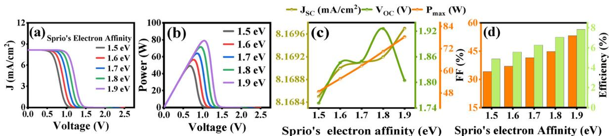
**Fig. 10** (a)  $J$ - $V$  curve and (b)  $P$ - $V$  curve of the TiO<sub>2</sub>/BFO/Spiro-OMeTAD solar cell. Effect of Spiro's electron affinity on (c)  $J_{sc}$ ,  $V_{oc}$ ,  $P_{max}$ , and (d) %FF and %efficiency.
