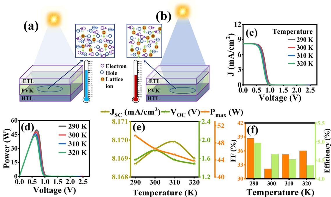
Fig. 11 (a) Higher temperature and (b) lower temperature effect on the device's internal environment. (c)  $J$ - $V$  curve and (d)  $P$ - $V$  curve of the  $\text{TiO}_2/\text{BFO}/\text{Spiro-OMeTAD}$  solar cell. Effect of temperature on (e)  $J_{\text{sc}}$ ,  $V_{\text{oc}}$ ,  $P_{\text{max}}$ , and (f) %FF and %efficiency.
