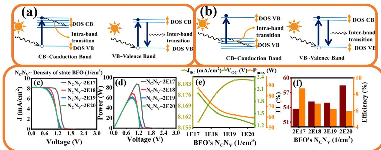
Fig. 6 (a and b) Schematic of the higher and lower density of states (DOS) in the conduction & valence bands ( $N_C N_V$ ) within the  $\text{BiFeO}_3$  (BFO) layer. (c)  $J$ - $V$  curve and (d)  $P$ - $V$  curve of the  $\text{TiO}_2/\text{BFO}/\text{Spiro-OMeTAD}$  solar cell. Effect of BFO's  $N_C N_V$  on (e)  $J_{sc}$ ,  $V_{oc}$ ,  $P_{max}$ , and (f) %FF and %efficiency.
