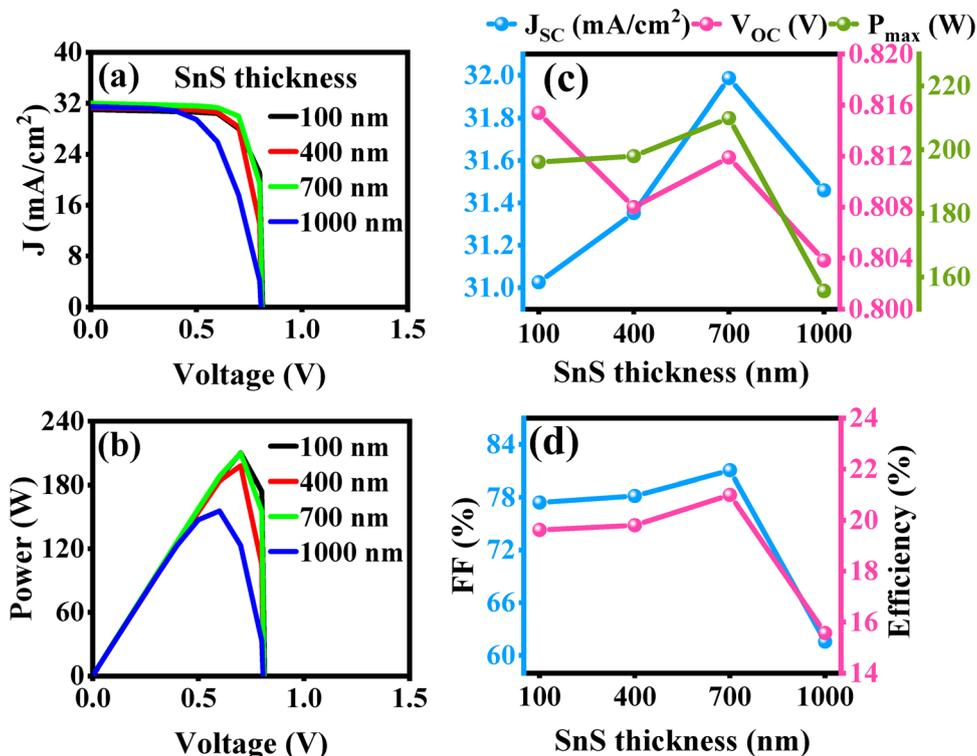
Fig. 12 (a)  $J$ - $V$  curve and (b)  $P$ - $V$  curve of the  $TiO_2/SnS/BFO/Spiro-OMeTAD$  solar cell. Effect of SnS's thickness on (c)  $J_{sc}$ ,  $V_{oc}$ ,  $P_{max}$ , and (d) %FF and %efficiency.
