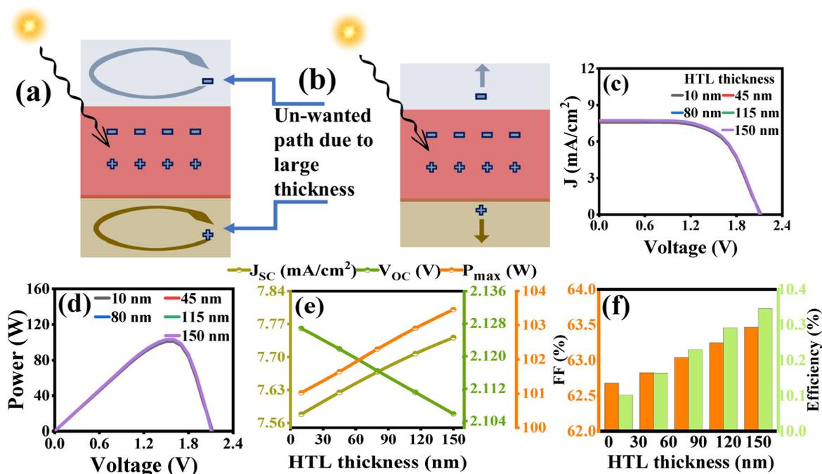
Fig. 5 (a and b) Schematic of the effect of thicker and thinner HTLs on the performance of solar cells. (c)  $J$ - $V$  curve and (d)  $P$ - $V$  curve of the  $\text{TiO}_2/\text{BFO}/\text{Spiro-OMeTAD}$  solar cell. Effect of the HTL's thickness variation on (e)  $J_{sc}$ ,  $V_{oc}$ ,  $P_{max}$ , and (f) %FF and %efficiency.
