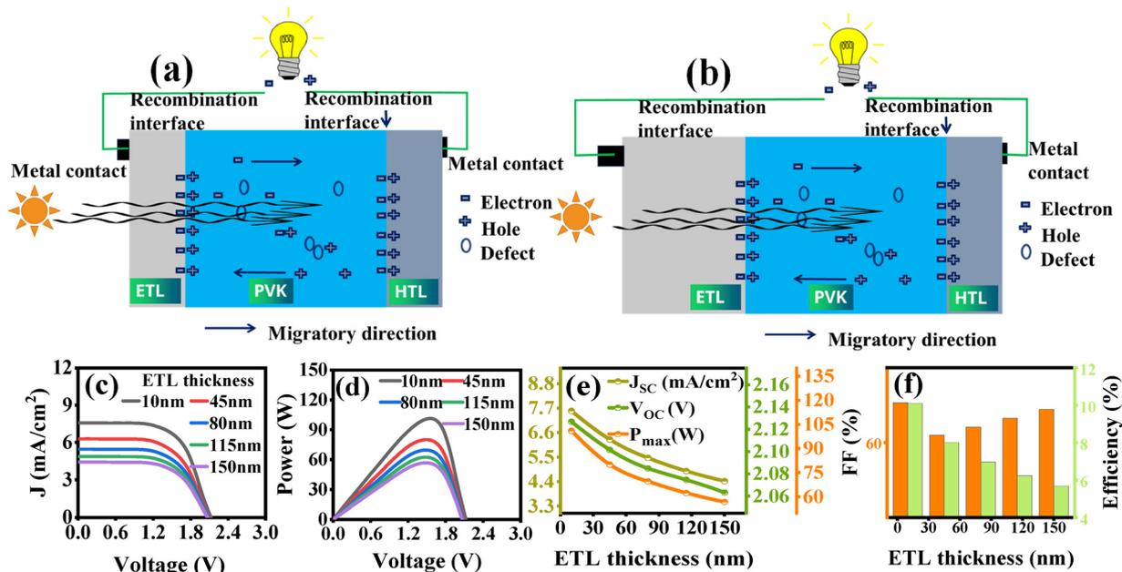
Fig. 4 Schematic of the effect of the ETL's thickness on the performance of solar cells: (a) thinner ETL and (b) thicker ETL. (c)  $J$ - $V$  curve and (d)  $P$ - $V$  curve of the  $\text{TiO}_2/\text{BFO}/\text{Spiro-OMeTAD}$  solar cell. Effect of the ETL's thickness variation on (e)  $J_{sc}$ ,  $V_{oc}$ ,  $P_{max}$ , and (f) %FF and %efficiency.
