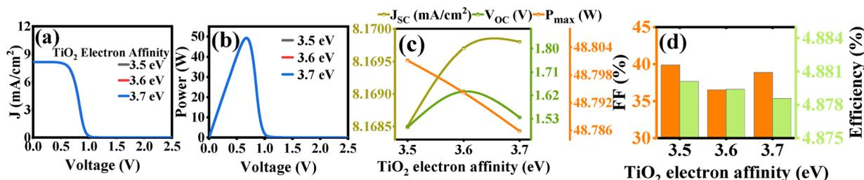
Fig. 9 (a)  $J$ - $V$  curve and (b)  $P$ - $V$  curve of the  $\text{TiO}_2/\text{BFO}/\text{Spiro-OMeTAD}$  solar cell. Effect of the electron affinity of  $\text{TiO}_2$  on (c)  $J_{\text{sc}}$ ,  $V_{\text{oc}}$ ,  $P_{\text{max}}$ , and (d) %FF and %efficiency.
