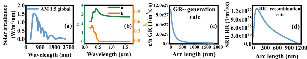
Fig. 1 (a) Solar spectrum, (b)  $n$  and  $k$  dependence on wavelength, (c) generation rate of  $e/h$  pairs inside the layers of solar cell, and (d) Shockley-Read-Hall recombination rate within the device.
