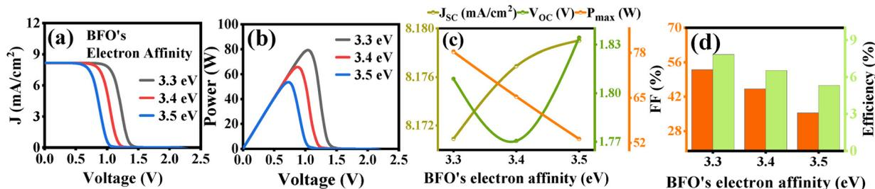
Fig. 8 (a)  $J$ - $V$  curve and (b)  $P$ - $V$  curve of the  $\text{TiO}_2/\text{BFO}/\text{Spiro-OMeTAD}$  solar cell. Effect of  $\text{BiFeO}_3$  (BFO)'s electron affinity on (c)  $J_{\text{sc}}$ ,  $V_{\text{oc}}$ ,  $P_{\text{max}}$ , and (d) %FF and %efficiency.
