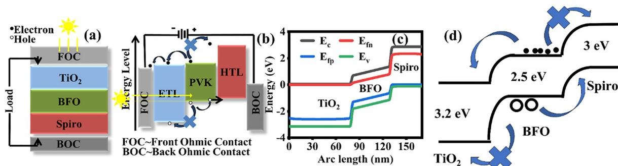
Fig. 2 (a) Solar cell's schematic, (b) schematic with energy levels, (c) energy-level variations vs. arc length, and (d) energy-band alignment of the  $TiO_2$ /BFO/Spiro-OMeTAD heterojunction solar cell for the transportation of charge carriers.
