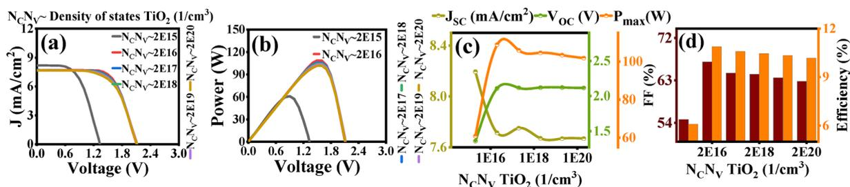
**Fig. 7** Effect of the density of states within the conduction and valence bands ( $N_{C,N_V}$ ) in the electron-transport layer (TiO<sub>2</sub>) on the solar cell performance. (a)  $J$ - $V$  curve and (b)  $P$ - $V$  curve of the TiO<sub>2</sub>/BFO/Spiro-OMeTAD solar cell. Effect of TiO<sub>2</sub>'s  $N_{C,N_V}$  on (c)  $J_{sc}$ ,  $V_{oc}$ ,  $P_{max}$ , and (d) FF and %efficiency.
