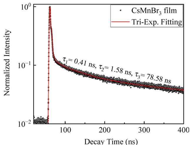
Fig. 4 Transient PL decay curves of the as-prepared CsMnBr<sub>3</sub> films fitted with the tri-exponential decay equation.
