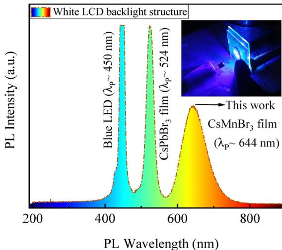
Fig. 7 PL response of the as-constructed white-emitting backlight structure showing distinct blue ( $\sim 450$  nm), green ( $\sim 524$  nm) and red ( $\sim 644$  nm) emission peaks with the inset depicting an optical image of the backlight structures under dark.
