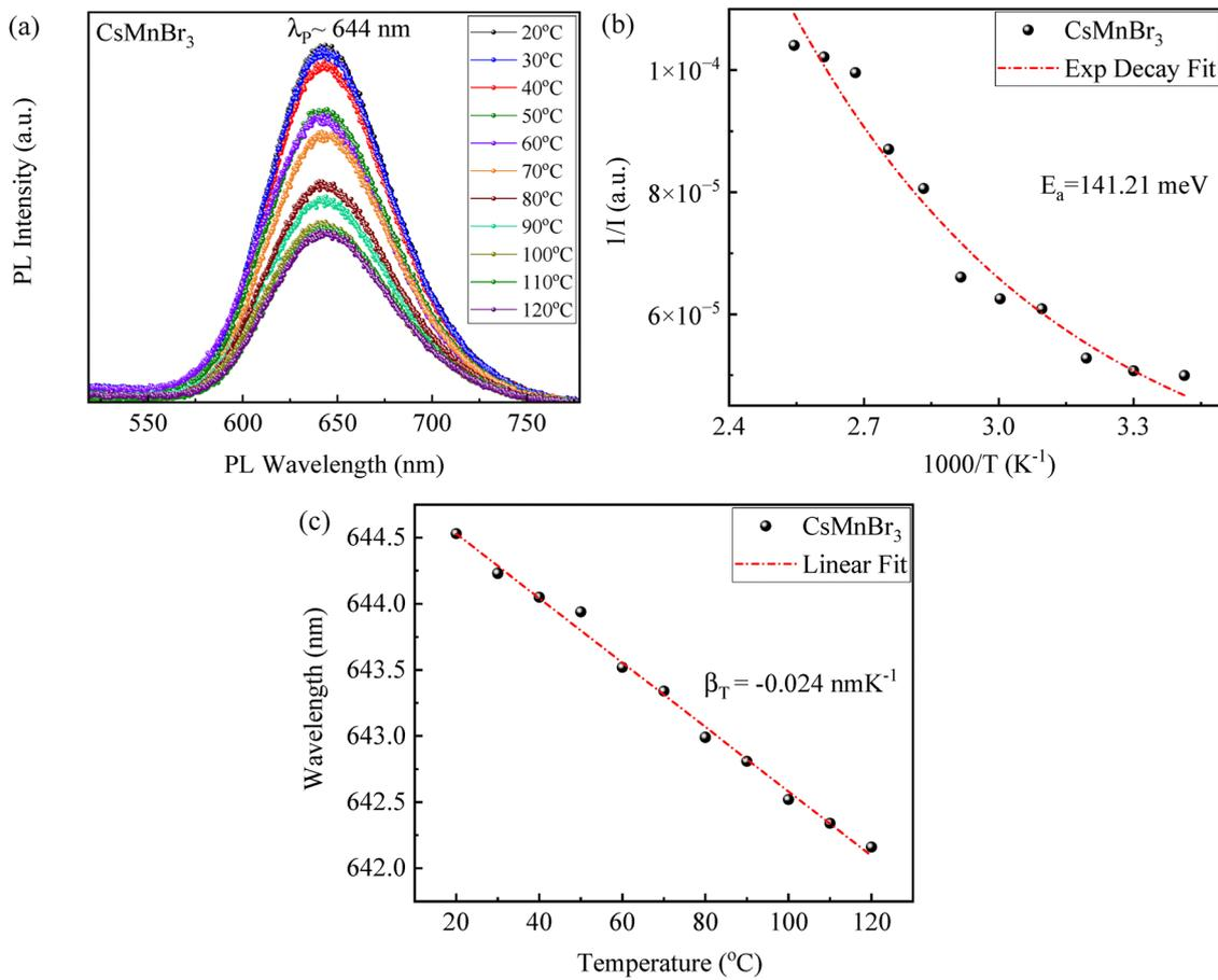
Fig. 5 (a) PL spectra of the as-prepared CsMnBr<sub>3</sub> films at different temperatures, (b) temperature dependence of PL peak intensity, and (c) temperature dependence of PL peak wavelength.
