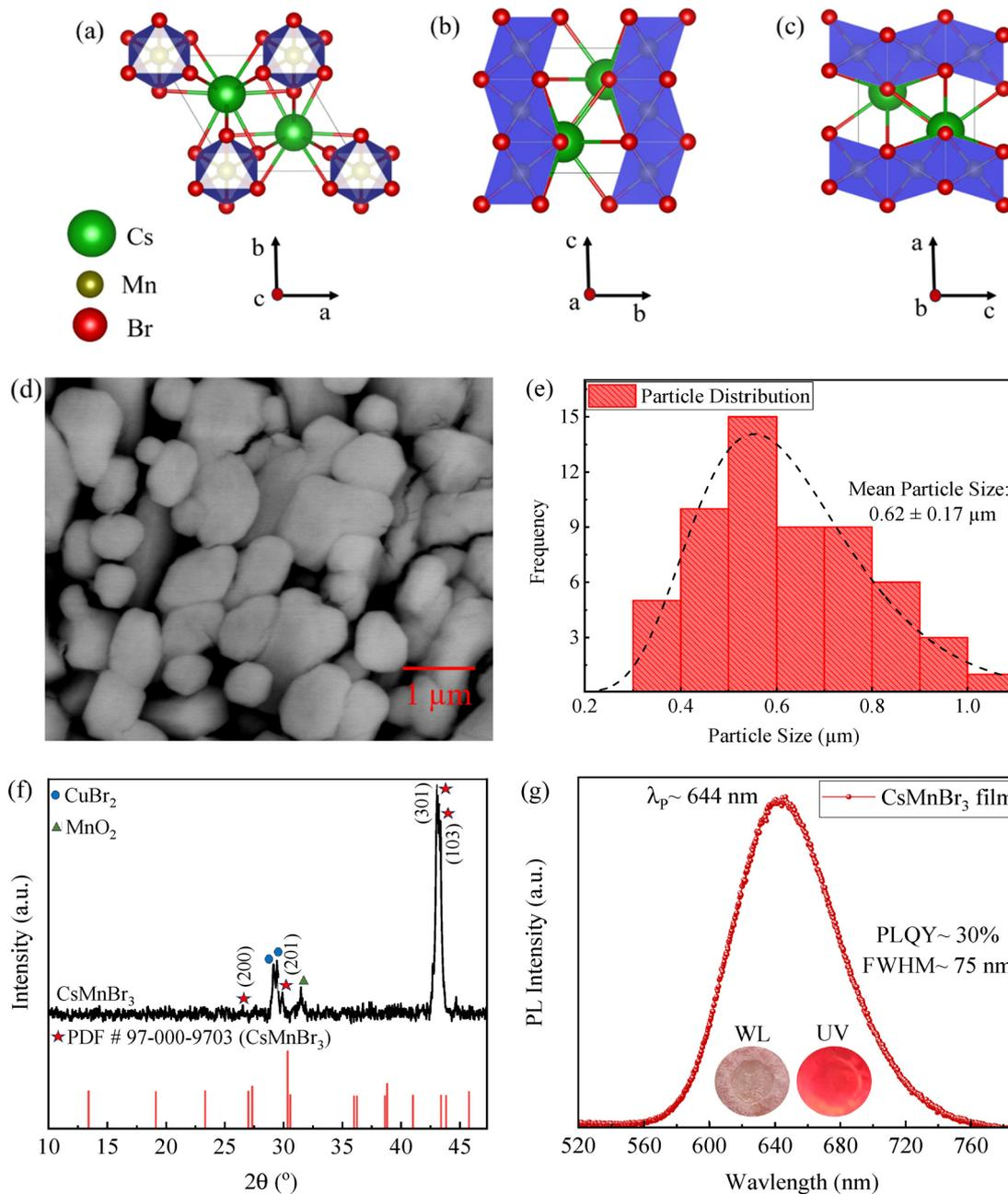
**Fig. 2** Crystal structure of  $\text{CsMnBr}_3$  projected along (a)  $c$ -axis, (b)  $a$ -axis, and (c)  $b$ -axis, (d) a SEM image of the as-prepared  $\text{CsMnBr}_3$  film, (e) histograms depicting the distribution of particle sizes, (f) XRD spectra of the as-prepared  $\text{CsMnBr}_3$  film, and (g) PL spectra of the as-prepared  $\text{CsMnBr}_3$  film with the inset showing optical images of the film under white and UV light ( $\sim 365$  nm), respectively.
