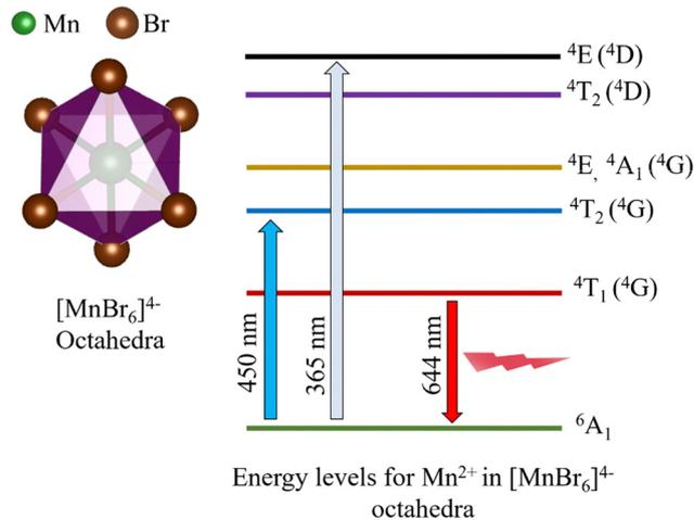
Fig. 8 Energy level diagram of octahedrally coordinated  $\text{Mn}^{2+}$  ions in CsMnBr<sub>3</sub>, depicting d-d transitions and the photoluminescence pathway for red emission ( $\sim 644$  nm).
