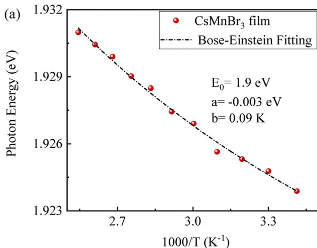
Fig. 9 Temperature dependence of photon energy for CsMnBr<sub>3</sub> films, fitted via the Bose–Einstein model.
