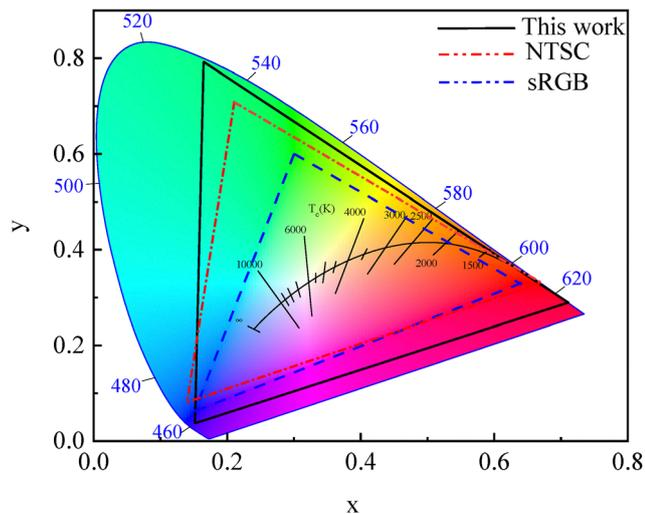
Fig. 11 CIE color gamut coverage of white emitting backlight structures from the as-prepared  $\text{CsMnBr}_3$  films ( $\lambda_p \sim 644$  nm).
