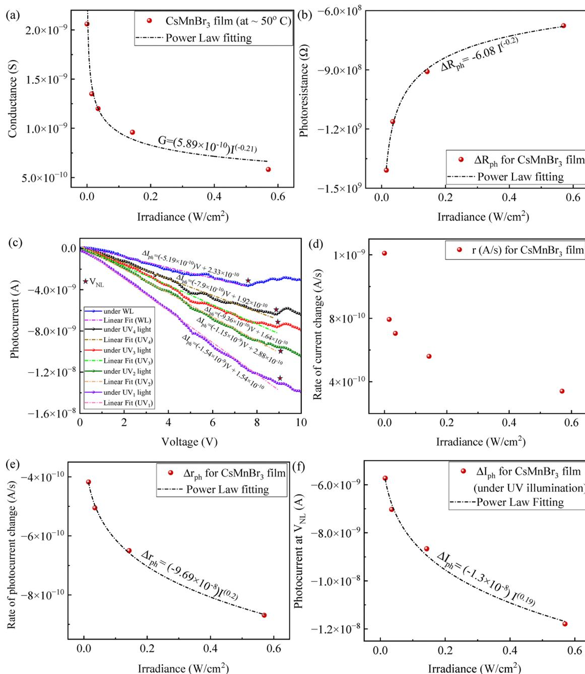
**Fig. 10** Electrical and photo-response characteristics of CsMnBr<sub>3</sub> films under UV (~365 nm) irradiation: (a) conductance as a function of UV irradiance, (b) photoresistance as a function of UV irradiance, (c) photocurrent–voltage characteristics, (d) change rate of current as a function of UV irradiance, (e) change rate of photocurrent as a function of irradiance, and (f) photocurrent at  $V_{NL}$  (onset of the non-linear region) as a function of irradiance.
