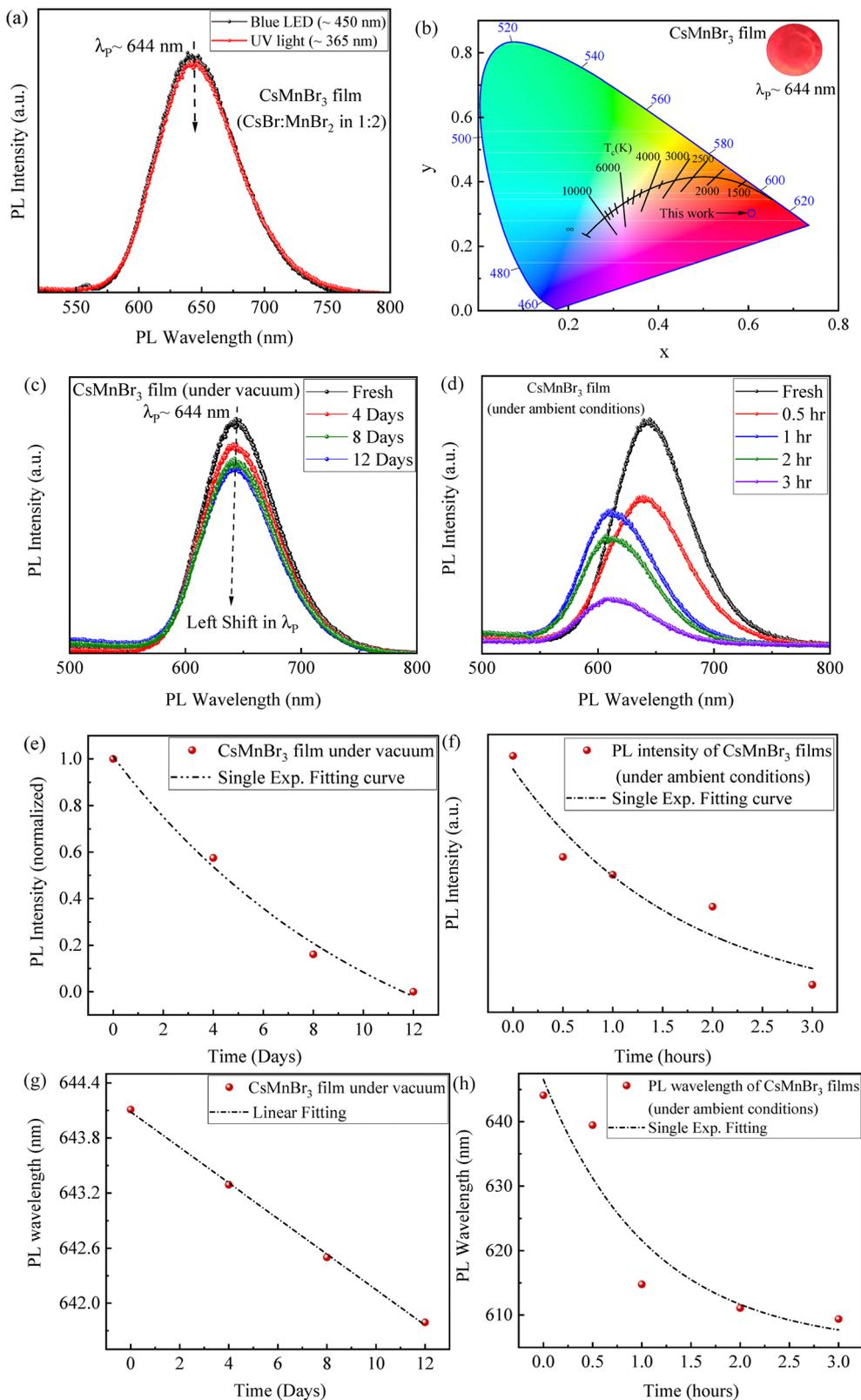
**Fig. 3** (a) PL spectra of CsMnBr<sub>3</sub> films under different excitation sources, (b) CIE chromaticity diagram of red-emitting CsMnBr<sub>3</sub> films, (c), (e) and (g) long-term stability curves of CsMnBr<sub>3</sub> films stored under vacuum conditions, and (d), (f) and (h) long-term stability curves of CsMnBr<sub>3</sub> films exposed to ambient conditions ( $T$ :  $\sim 17$  °C, RH:  $\sim 65\%$ ).
