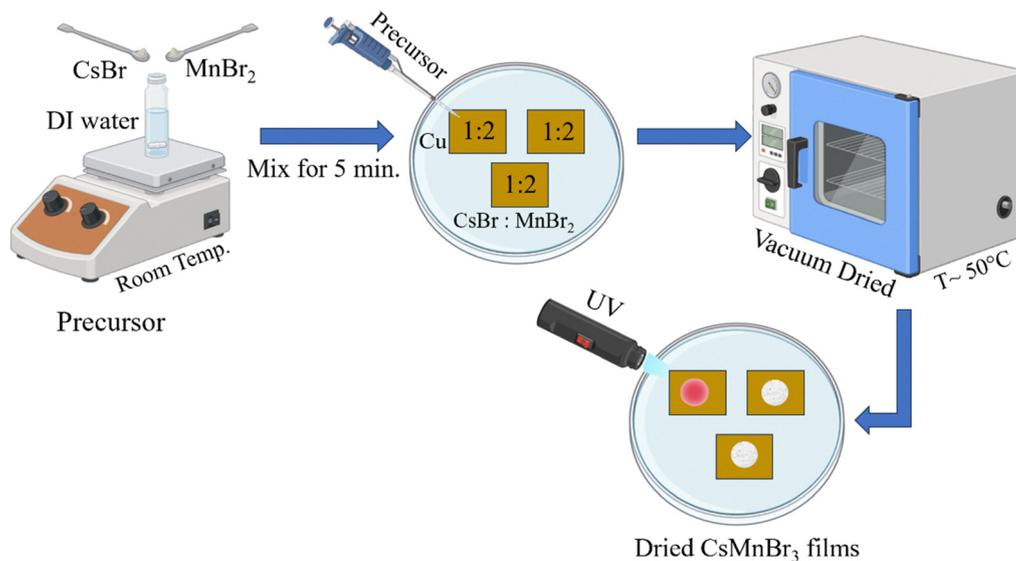
Fig. 1 Schematic depicting the synthesis route of CsMnBr<sub>3</sub> films via an aqueous solution of CsBr and MnBr<sub>2</sub> in a 1 : 2 molar ratio.
