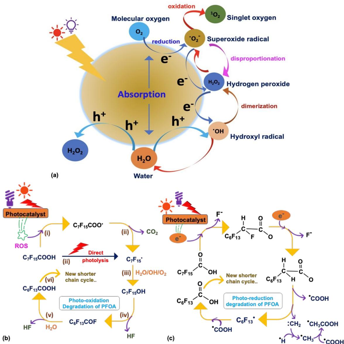
**Figure 4.** (a) General photocatalytic mechanism depicting electron–hole pair formation and subsequent redox reactions; (b) General pathway of photo-oxidative degradation of PFOA; (c) Typical pathway of photo-reductive degradation of PFOA.
