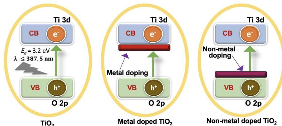
**Figure 7.** Schematic illustrating the effects of metal and non-metal dopants on the properties and activity of TiO<sub>2</sub>-based photocatalysts.
