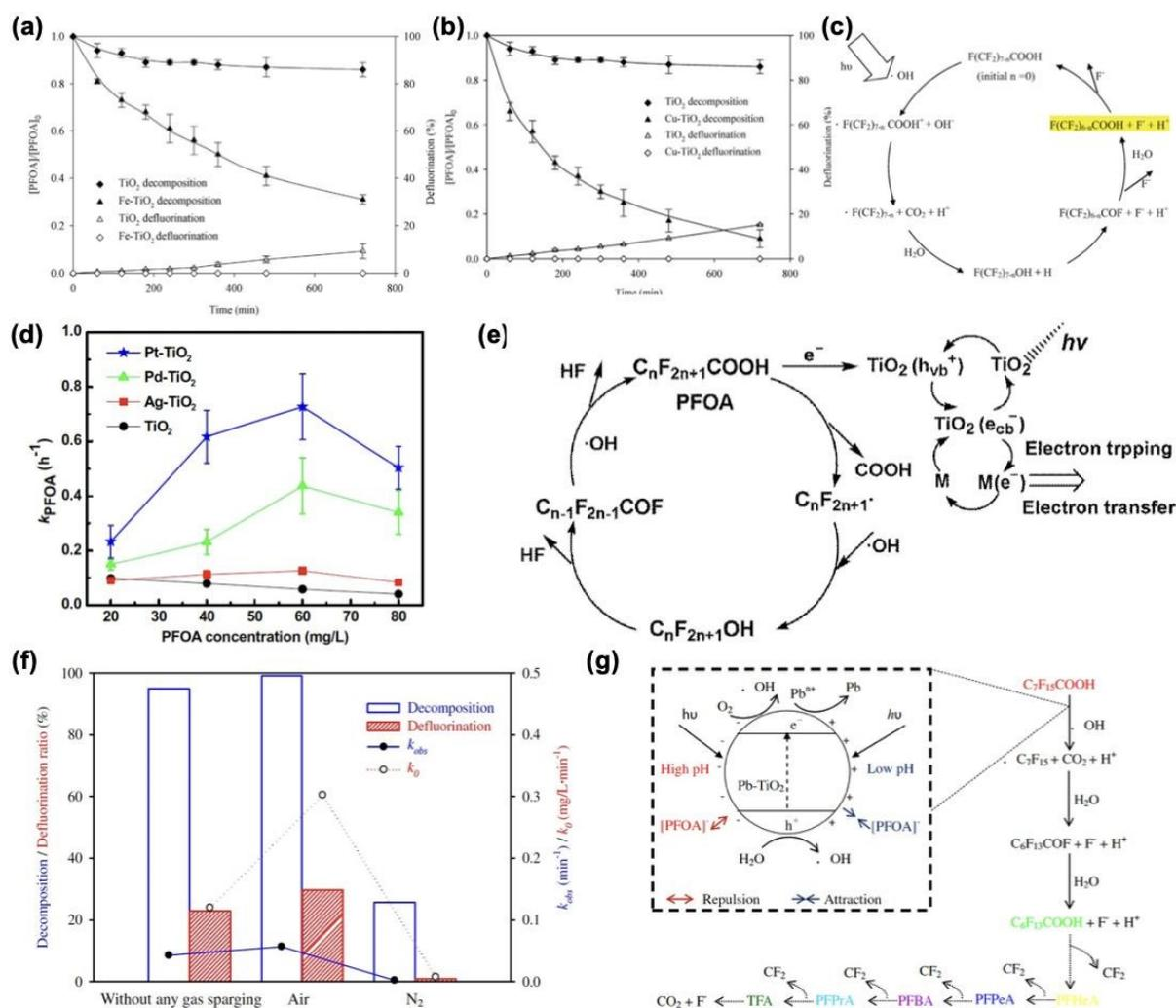
**Figure 8.** Photocatalytic degradation of PFOA using TiO<sub>2</sub>-based materials: (a) Comparison of degradation and defluorination efficiency: bare TiO<sub>2</sub> (~14% degradation in 12 h), Fe-TiO<sub>2</sub> (~69% degradation, 9% defluorination), (b) Cu-TiO<sub>2</sub> (~91% degradation, 19% defluorination), (c) Schematic of PFOA
