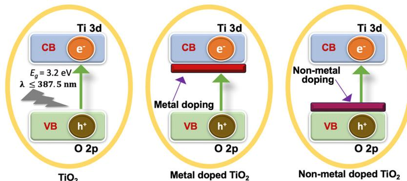
Fig. 7 Schematic illustrating the effects of metal and non-metal dopants on the properties and activity of TiO<sub>2</sub>-based photocatalysts.
