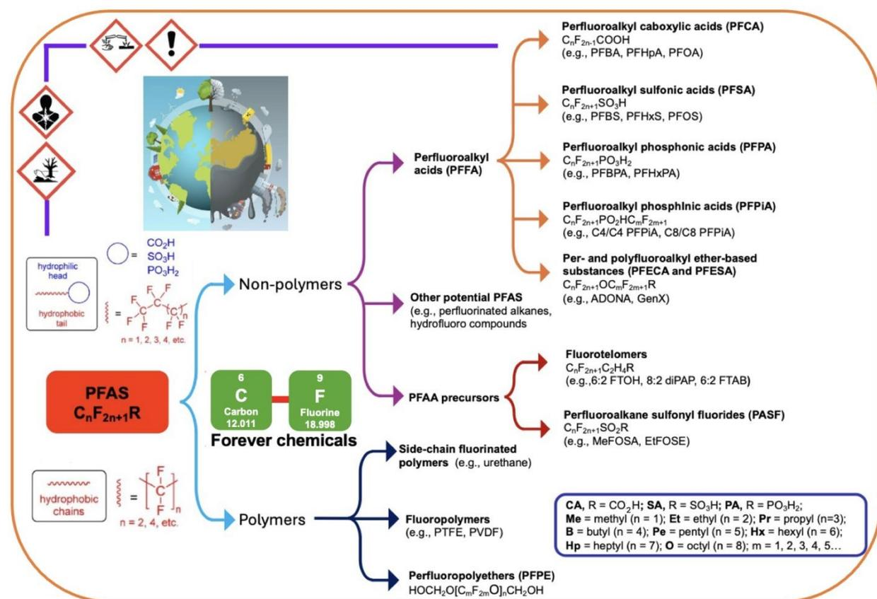
**Figure 2.** Classification of PFAS based on structural features, categorized into polymeric and non-polymeric groups.
