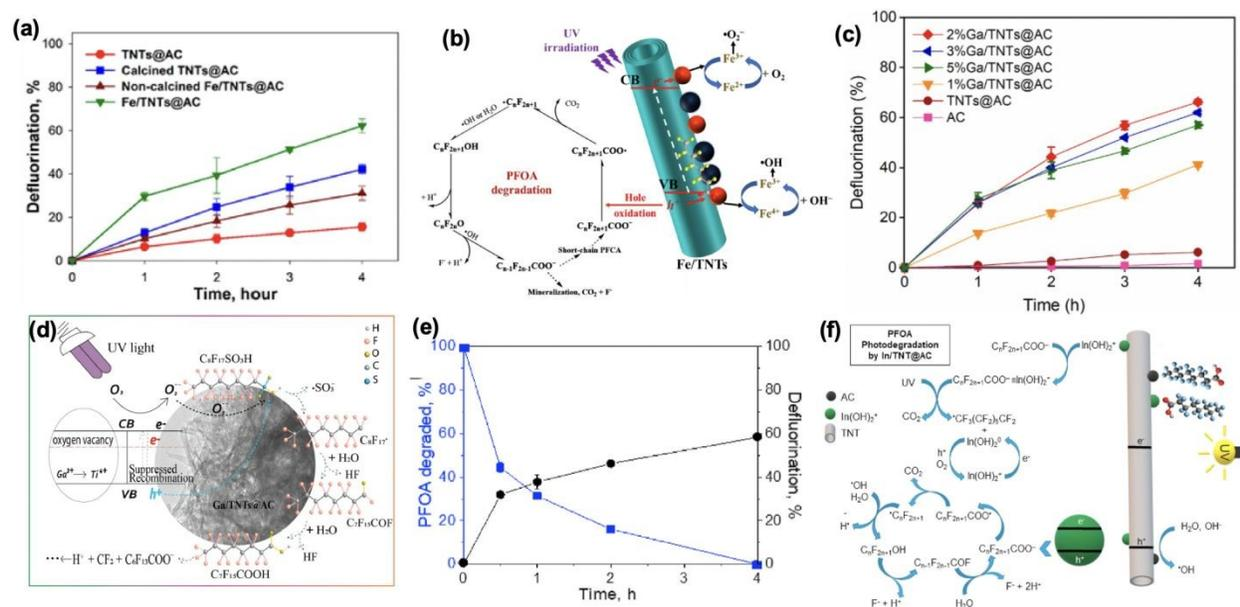
**Figure 11.** (a) Photocatalytic defluorination of PFOA, showing  $\sim 62\%$  conversion of organic fluorine to F<sup>-</sup> by Fe/TNTs@AC under UV irradiation, significantly higher than TNTs@AC and other controls, (b) Proposed photocatalytic degradation mechanism of PFOA on iron (hydr)oxide-impregnated nanoparticles under UV irradiation, showing adsorption, hole/electron generation, radical formation, and stepwise defluorination
