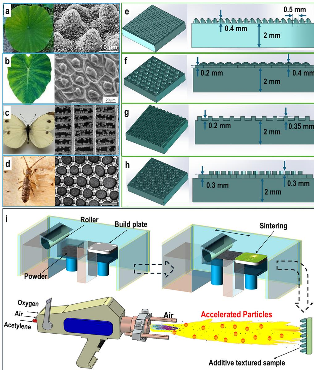
**Fig. 1** Fabrication process of bioinspired superhydrophobic coatings. (a)–(d) Microstructures of a lotus leaf (*Nelumbo nucifera*), taro leaf (*Colocasia esculenta*), butterfly wings (*Pieris canidia*), and slender springtail (*Entomobrya nivalis*). (e)–(h) 3D-designed macrographs through SolidWorks, and (i) schematic illustration showing the fabrication of superhydrophobic surfaces through additive manufacturing and flame spraying.
