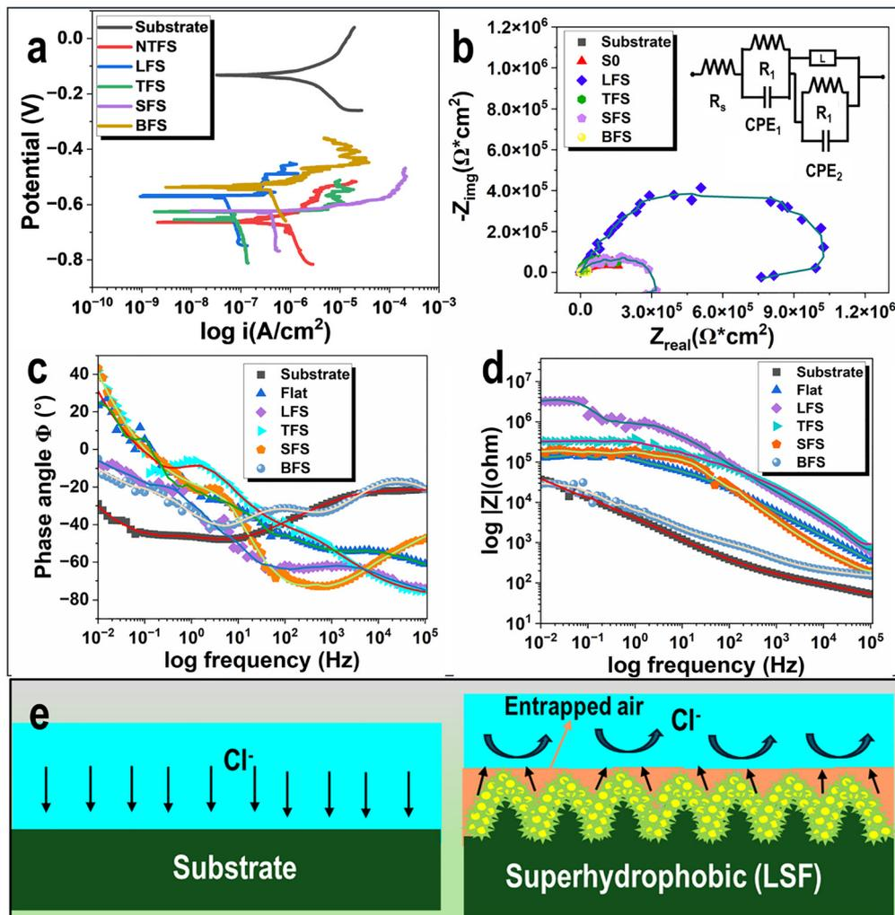
Fig. 7 The corrosion behavior of the substrate, and the NTFS, LFS, TFS, SFS, and BSF superhydrophobic samples is depicted through (a) potentiodynamic polarization results and (b) Nyquist plots with electrical equivalent circuit in the inset, and (c) and (d) Bode plots. (e) Schematic explaining the interaction of aggressive chloride ions with the substrate and superhydrophobic sample where entrapped air acts as an insulating medium for ion exchange.
