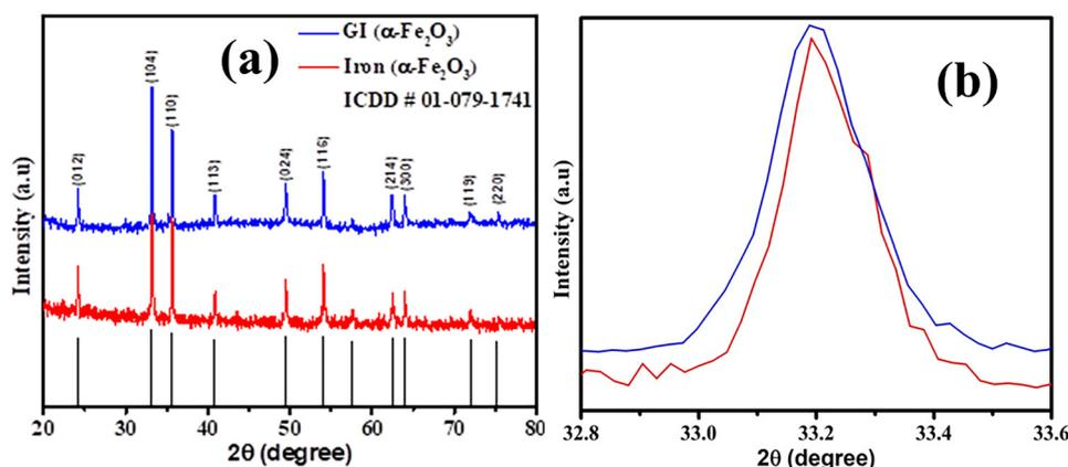
**Fig. 1** XRD patterns of the (a) GI-oxide NPs and the pure iron-oxide NPs and (b) zoomed in view of the overlapping peaks.
