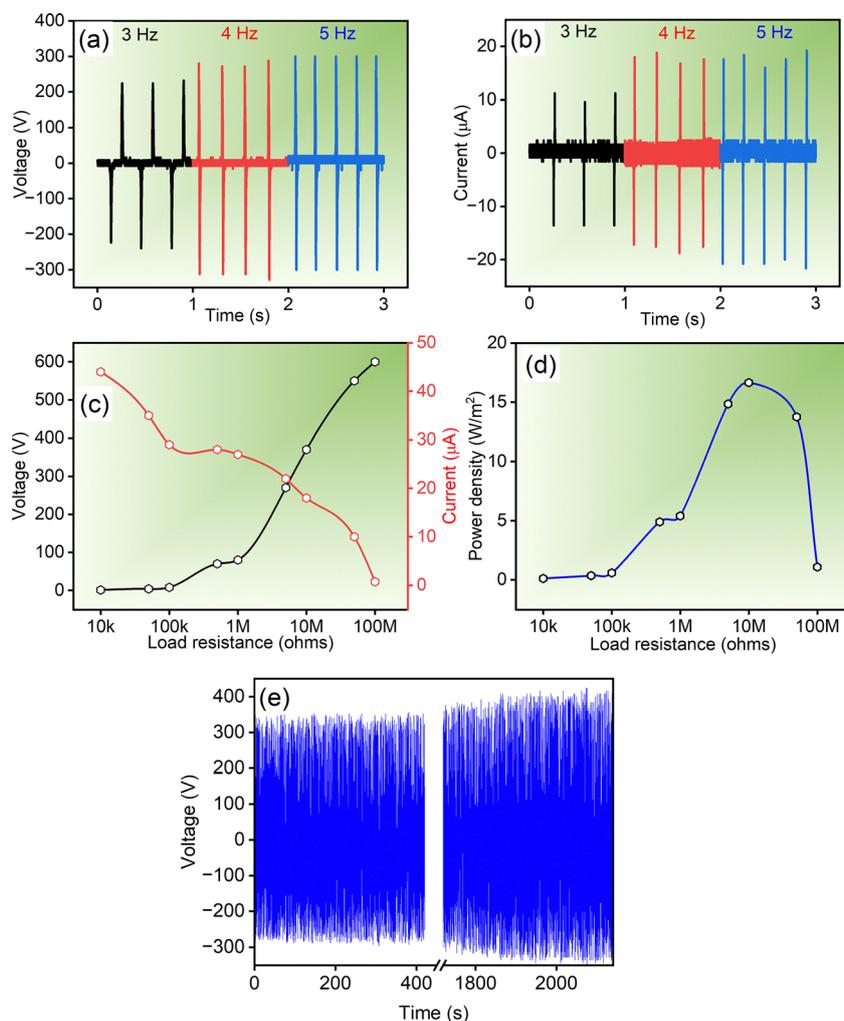
Fig. 6 (a)  $V_{oc}$  and (b)  $I_{sc}$  of fabricated TENGs using a linear-motor-based contact-separation mechanism. The measured (c)  $V_{oc}$  and  $I_{sc}$ , (d) power density on the external load resistance in the range of 10 k $\Omega$  to 100 M $\Omega$  of MC-TENG, (e) Stability measurement test of MC-TENG for more than 10 000 cycles.
