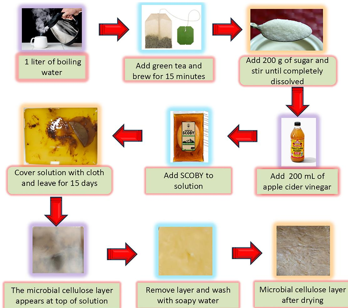
Fig. 1 Flow chart depicting the detailed synthesis of microbial cellulose.
