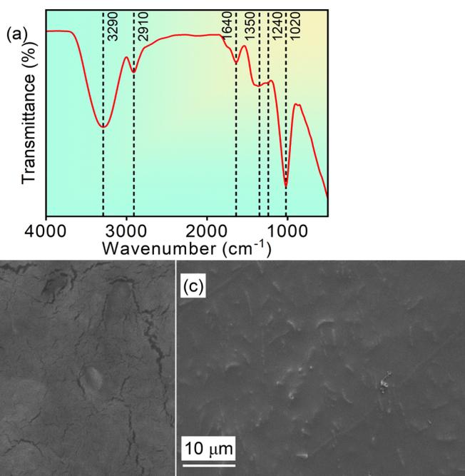
Fig. 3 (a) FTIR spectra and (b) & (c) Surface micrographs of the microbial cellulose film.
